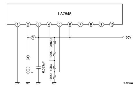
In the circuit in figure 2 with the output from pin 2 absorbed by an electronic load and read the value shown by the voltage meter (V) when the current meter (A) reads 1.1A.
