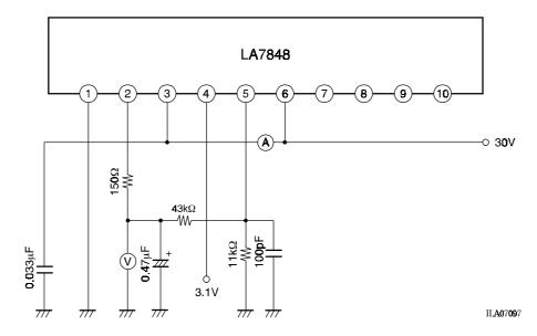
In the circuit in figure 5, read the value shown by the current meter (A). In the circuit in figure 5, read the value shown by the voltage meter (V).
