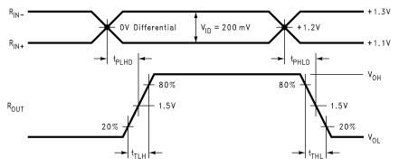
Figure 3. Receiver Propagation Delay and Transition Time Waveforms
