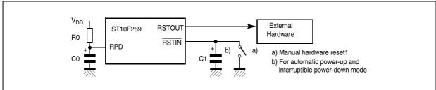
Figure 59. External Reset Hardware Circuitry
