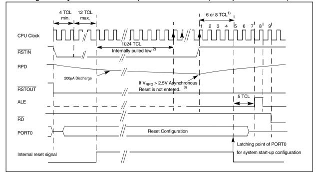
Figure 55. Synchronous Reset Sequence External Fetch (RSTIN pulse > 1040 TCL)
