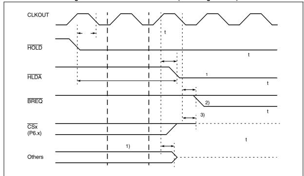
Figure 78. External Bus Arbitration (Releasing the Bus)
