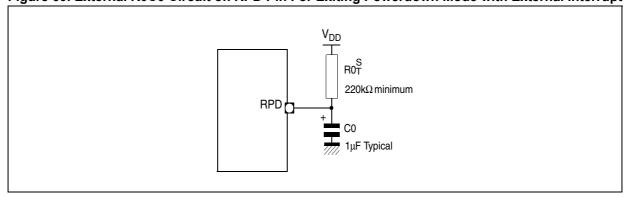
To exit Power Down mode with an external interrupt, an EXxIN (x = 7...0) pin has to be asserted for at least 40 ns.
