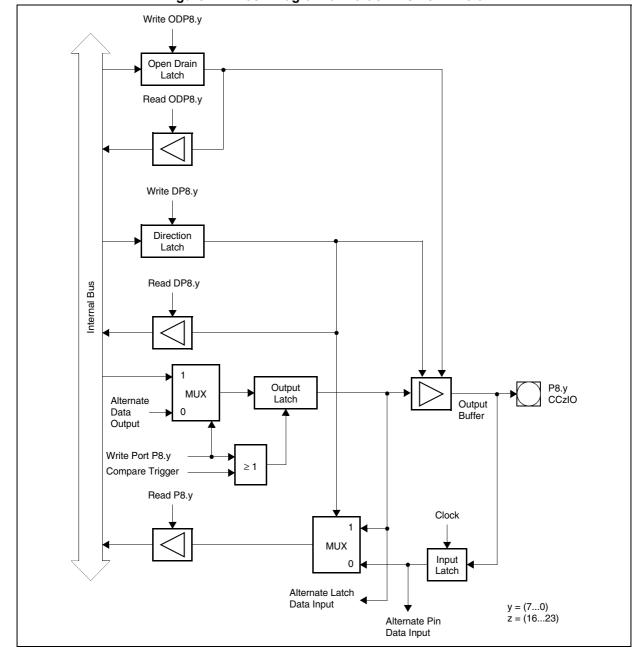
Figure 42. Block Diagram of Port 8 Pins P8.7...P8.0
