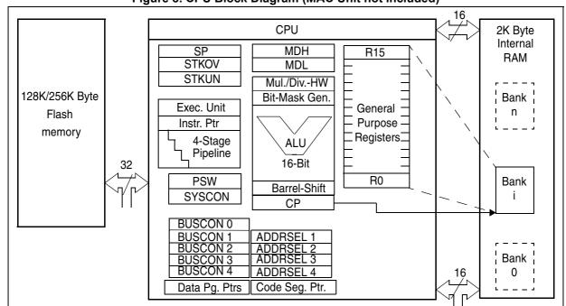
Figure 8. CPU Block Diagram (MAC Unit not included)
