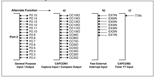
Figure 24. PORT2 I/O and Alternate Functions
