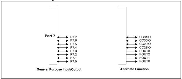
The structure of Port 7 differs in the way the output latches are connected to the internal bus and to the pin driver. Pins P7.3...P7.0 (POUT3...POUT0) EXOR the alternate data output with the port latch output, which allows to use the alternate data directly or inverted at the pin driver.
