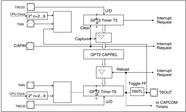
Figure 15. Block Diagram of GPT2
