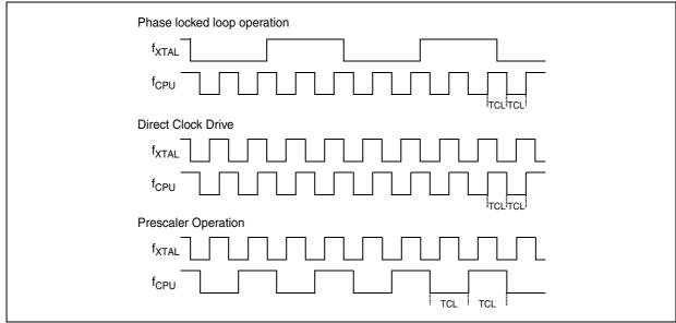
Figure 66. Generation Mechanisms for the CPU Clock
