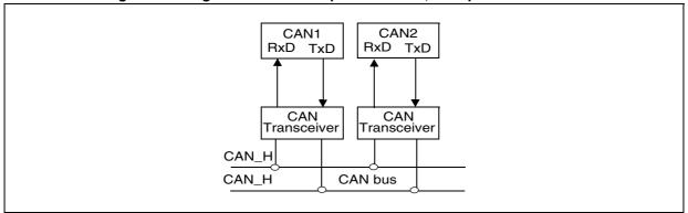
The ST10F269 also supports single CAN Bus multiple (dual) interfaces using the open drain option of the CANx\_TxD output as shown in *Figure 47*. Thanks to the OR-Wired Connection, only one transceiver is required. In this case the design of the application must take in account the wire length and the noise environment.
