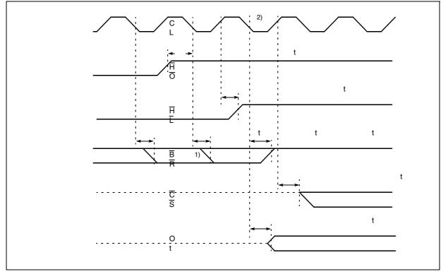
Figure 79. External Bus Arbitration (Regaining the Bus)
