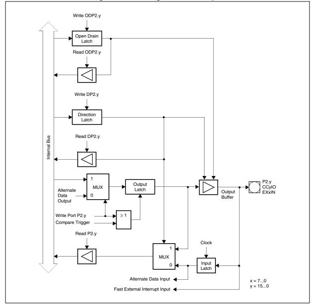
Figure 25. Block Diagram of a PORT2 pin
