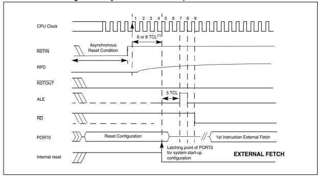
Figure 53. Asynchronous Reset Sequence External Fetch
