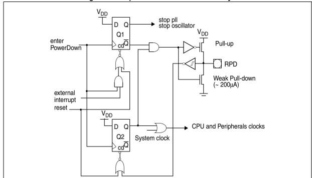
Figure 61. Simplified Powerdown Exit Circuitry
