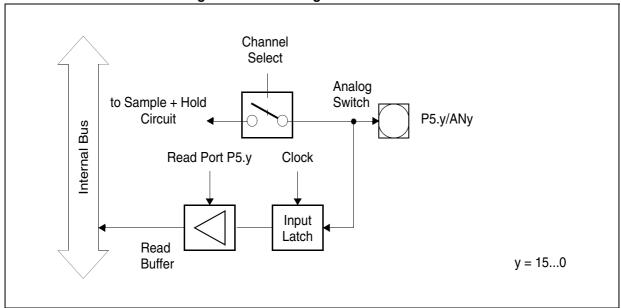
Figure 34. Block Diagram of a Port 5 Pin
