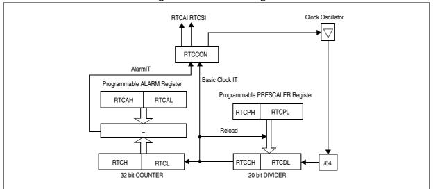
Figure 50. RTC Block Diagram
