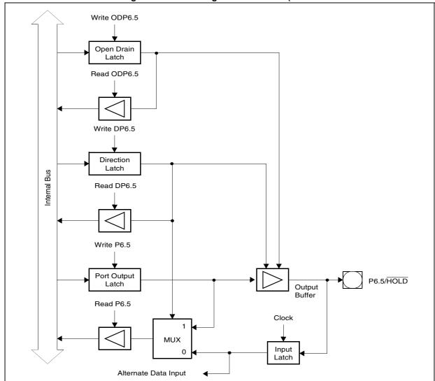
Figure 37. Block Diagram of Pin P6.5 (HOLD
