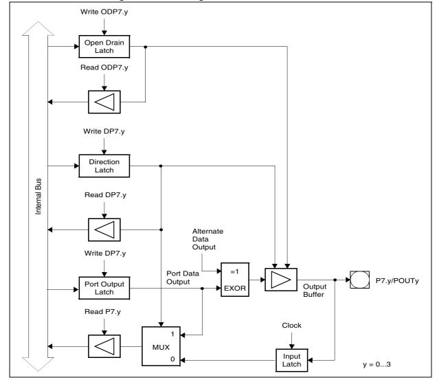
Figure 39. Block Diagram of Port 7 Pins P7.3...P7.0
