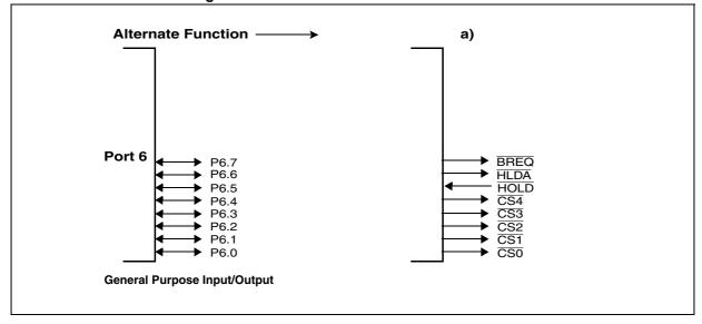
Figure 35. PORT6 I/O and Alternate Functions
