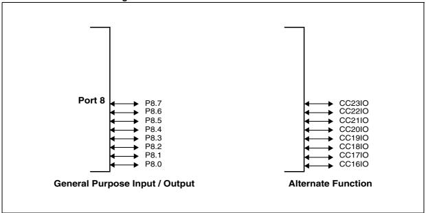
The structure of Port 8 differs in the way the output latches are connected to the internal bus and to the pin driver (see *Figure 42*). Pins P8.7...P8.0 (CC23IO...CC16IO) combine internal bus data and alternate data output before the port latch input, as do the Port 2 pins
