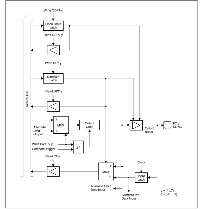
Figure 40. Block Diagram of Port 7 Pins P7.7...P7.
