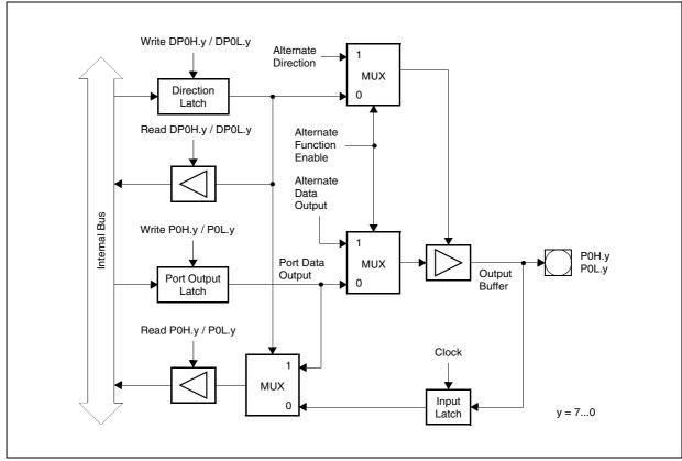
Figure 21. Block Diagram of a PORT0 pin
