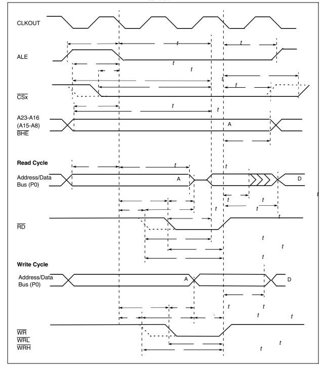
Figure 70. External Memory Cycle: Multiplexed Bus, With/Without Read/Write Delay, Extended ALE
