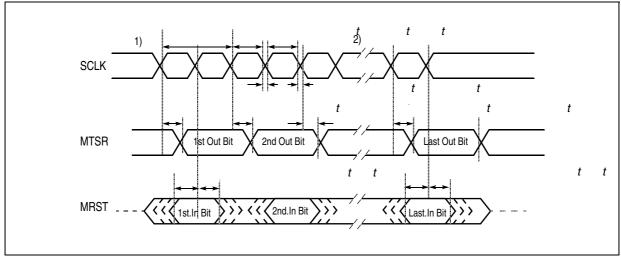
Figure 80. SSC Master Timing
