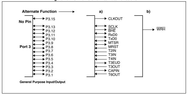
The structure of the Port 3 pins depends on their alternate function (see Figure 27 and Figure 28). When the on-chip peripheral associated with a Port 3 pin is configured to use the alternate input function, it reads the input latch, which represents the state of the pin, via the line labeled "Alternate Data Input". Port 3 pins with alternate input functions are: T0IN, T2IN, T3IN, T4IN, T3EUD and CAPIN.
