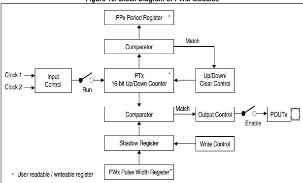
Figure 16. Block Diagram of PWM Modules
