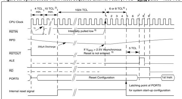
Figure 56. Synchronous Warm Reset Sequence External Fetch (4 TCL < RSTIN pulse < 1038 TCL
