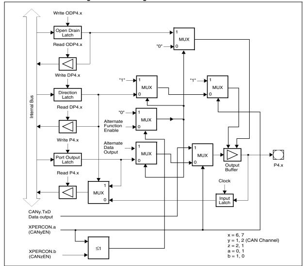
Figure 32. Block Diagram of P4.6 and P4.7 Pins
