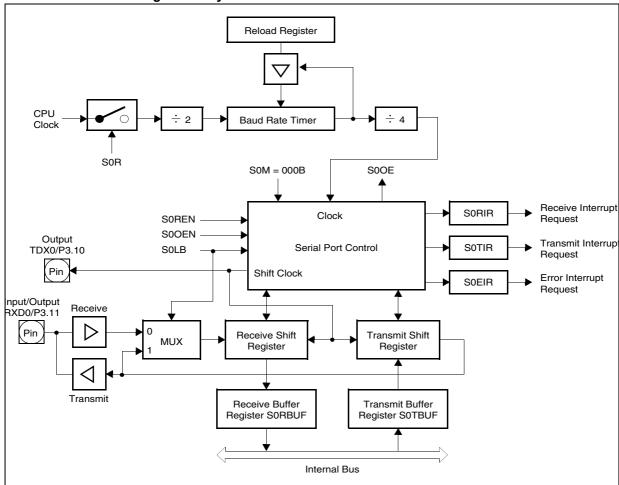
Figure 44. Synchronous Mode of Serial Channel ASC0
