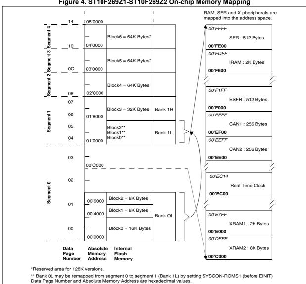
Figure 4. ST10F269Z1-ST10F269Z2 On-chip Memory Mapping
