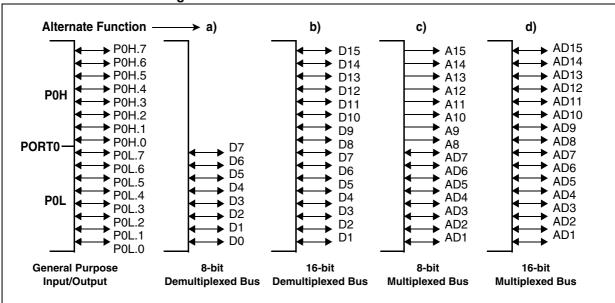
Figure 20. PORT0 I/O and Alternate Functions
