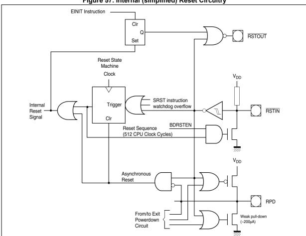
Figure 57. Internal (simplified) Reset Circuitry
