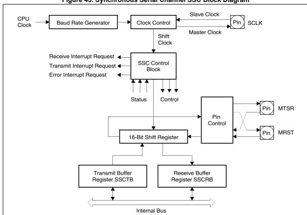
Figure 45. Synchronous Serial Channel SSC Block Diagram
