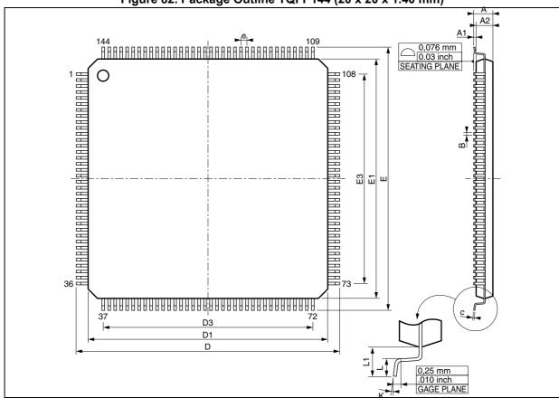
Figure 82. Package Outline TQFP144 (20 x 20 x 1.40 mm)
