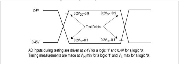
Figure 65. Float Waveforms
