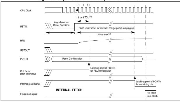
Figure 54. Asynchronous Reset Sequence Internal Fetch
