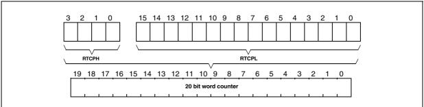
The value stored into RTCPH, RTCPL is called RTCP (coded on 20-bit). The dividing ratio of the Prescaler divider is: ratio = 64 x (RTCP)
