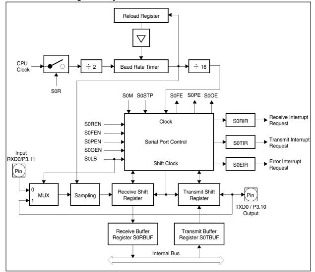
Figure 43. Asynchronous Mode of Serial Channel ASC0
