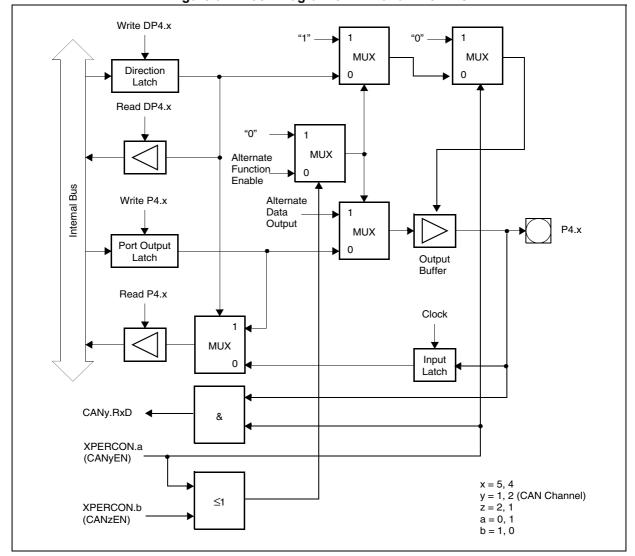
Figure 31. Block Diagram of P4.4 and P4.5 Pins
