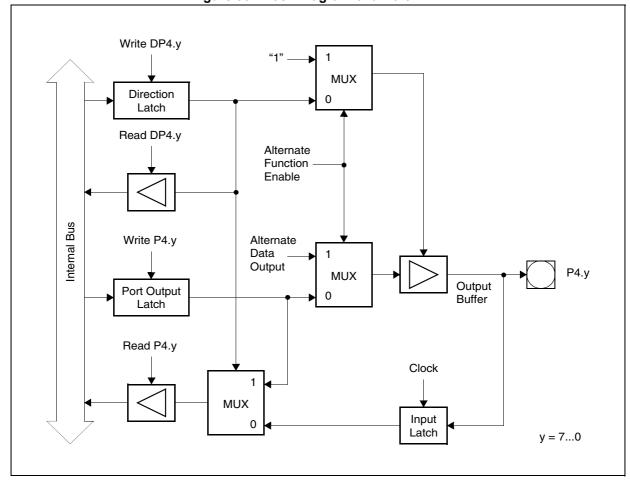
Figure 30. Block Diagram of a Port 4 Pin
