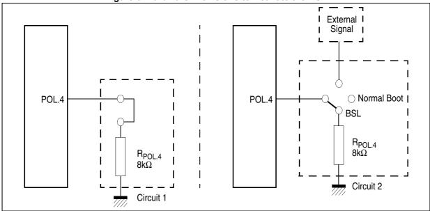
Figure 6. Hardware Provisions to Activate the BSL
