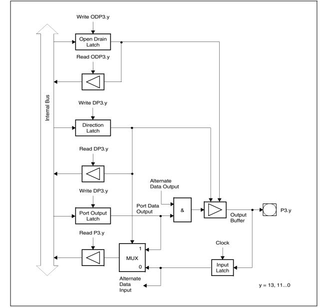
Figure 27. Block Diagram of Port 3 Pin with Alternate Input or Alternate Output Function
