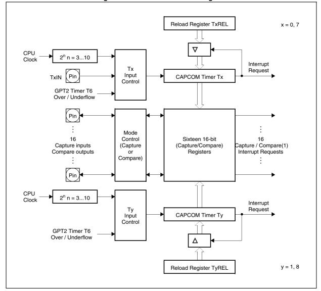
Figure 11. CAPCOM Unit Block Diagram
