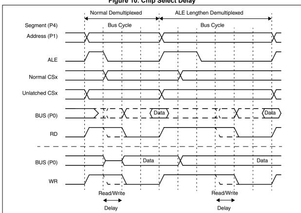
Figure 10. Chip Select Delay
