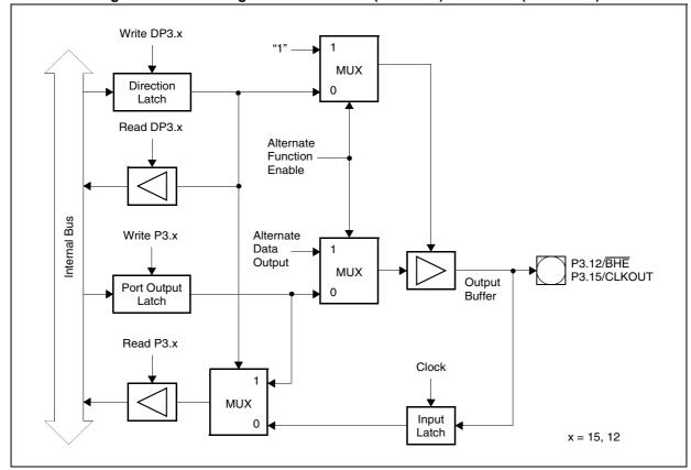
Figure 28. Block Diagram of Pins P3.15 (CLKOUT) and P3.12 (BHE/WRH)
