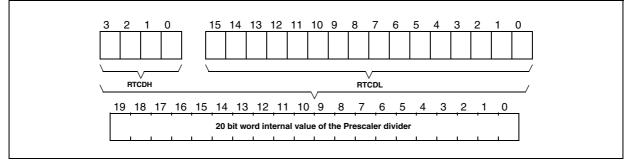
Bit 15 to bit 4 of RTCPH and RTCDH are not used. When reading, the return value of those bit will be zeros.
