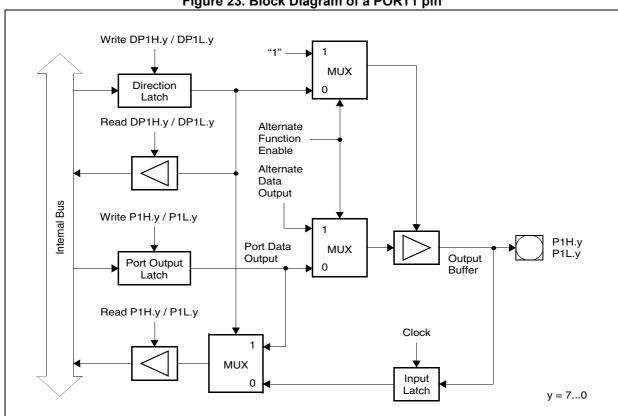
Figure 23. Block Diagram of a PORT1 pin
