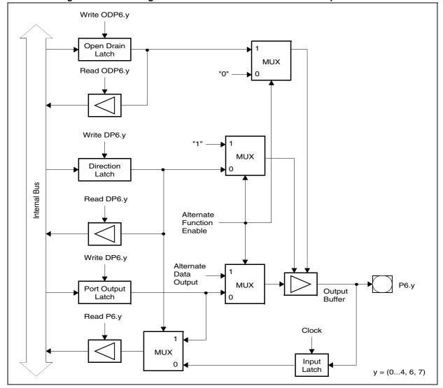
Figure 36. Block Diagram of Port 6 Pins with an Alternate Output Function
