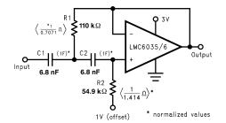
Figure 48. 2 Pole, 300Hz, Sallen and Key, High-Pass Filter
