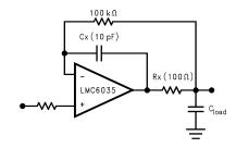
Figure 52. Rx, Cx Improve Capacitive Load Tolerance
