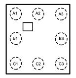
Figure 1. 8-Bump DSBGA Package (Bump Side Down) See Package Number YZR0008
