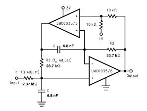
Figure 49. 2 Pole, 1kHz Active, Bandpass Filter
