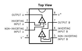
Figure 54. 8-Pin SOIC or VSSOP Package See Package Number D0008A or DGK0008A
