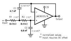
Figure 47. 2-Pole, 3kHz, Active, Sallen and Key, Lowpass Filter with Butterworth Response
