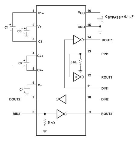
$^\dagger$  C3 can be connected to V<sub>CC</sub> or GND.
