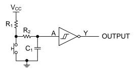
Figure 8. Push Button Debounce Circuit Schematic
