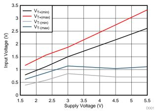
Figure 9. Interpolated Threshold Voltages vs.  $V_{CC}$
