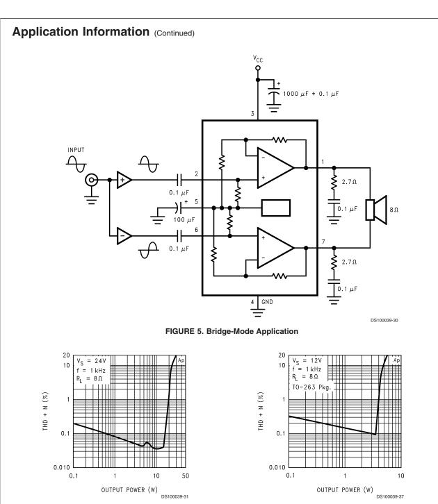
FIGURE 6. THD+N vs. POUT for Bridge-Mode Application
