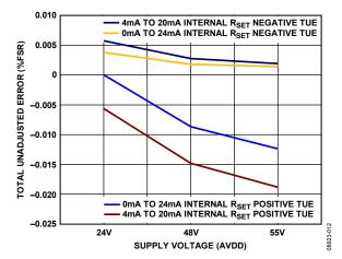
Figure 12. Total Unadjusted Error Current Mode, Internal R<sub>SET</sub> Sense Resistor
