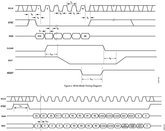
Figure 3. Readback Mode Timing Diagram
