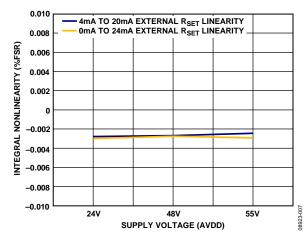
Figure 7. Integral Nonlinearity Current Mode, External R<sub>SET</sub> Sense Resistor
