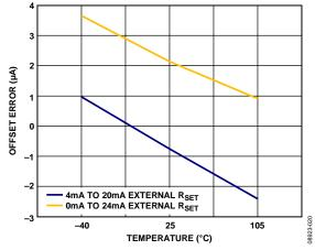
Figure 20. Offset Error vs. Temperature, External R<sub>SET</sub> Sense Resistor
