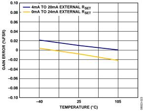
Figure 23. Gain Error vs. Temperature, External R<sub>SET</sub> Sense Resistor
