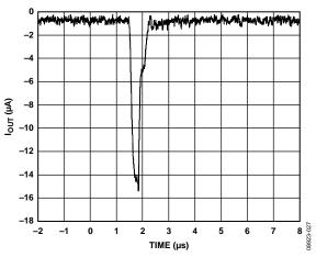
Figure 27. Output Current vs. Time on Output Enable, 0 mA to 24 mA Range
