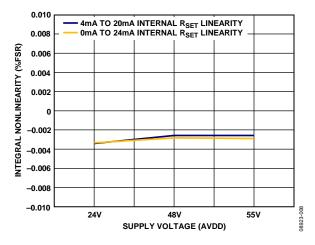
Figure 8. Integral Nonlinearity Current Mode, Internal R<sub>SET</sub> Sense Resistor
