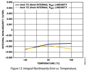
Internal R<sub>SET</sub> Sense Resistor
