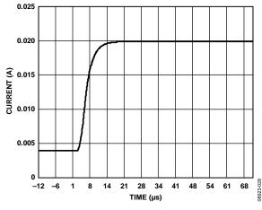
Figure 28. 4 mA to 20 mA Output Current Step
