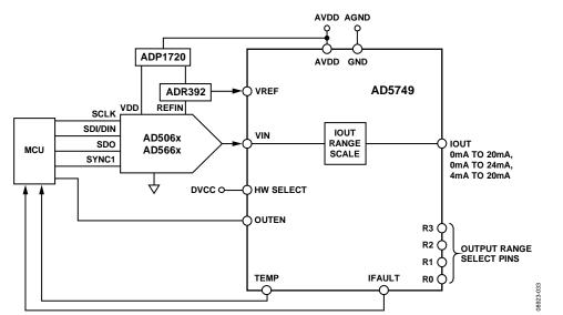
Figure 32. Typical System Configuration in Hardware Mode Using Internal DAC Reference (Pull-Up Resistors Not Shown for Open-Drain Outputs)
