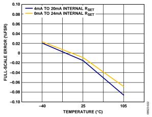
Figure 22. Full-Scale Error vs. Temperature, Internal R<sub>SET</sub> Sense Resistor
