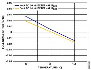
Figure 21. Full-Scale Error vs. Temperature, External R<sub>SET</sub> Sense Resistor
