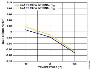
Figure 24. Gain Error vs. Temperature, Internal R<sub>SET</sub> Sense Resistor
