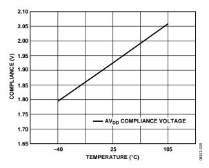
Figure 25. Output Compliance vs. Temperature Tested When  $I_{OUT} = 10.8$  mA, 0 mA to 24 mA Range Selected
