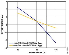
Figure 19. Offset Error vs. Temperature, Internal R<sub>SET</sub> Sense Resistor
