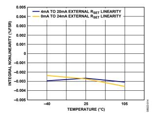
Figure 14. Integral Nonlinearity Error vs. Temperature, External R<sub>SET</sub> Sense Resistor
