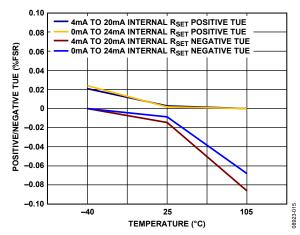
Figure 15. Total Unadjusted Error vs. Temperature, Internal R<sub>SET</sub> Sense Resistor
