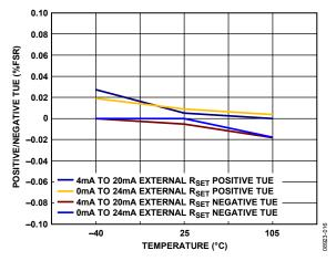
Figure 16. Total Unadjusted Error vs. Temperature, External R<sub>SET</sub> Sense Resistor
