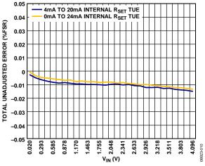
Figure 10. Total Unadjusted Error vs. VIN, Internal RSET Resistor
