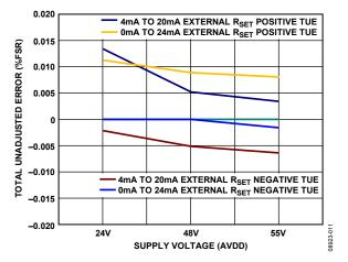
Figure 11. Total Unadjusted Error Current Mode, External R<sub>SET</sub> Sense Resistor
