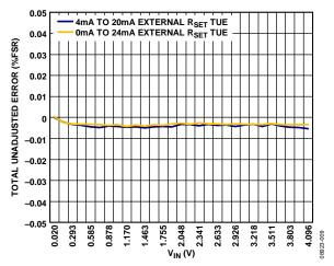
Figure 9. Total Unadjusted Error vs. V<sub>IN</sub>, External R<sub>SET</sub> Resistor
