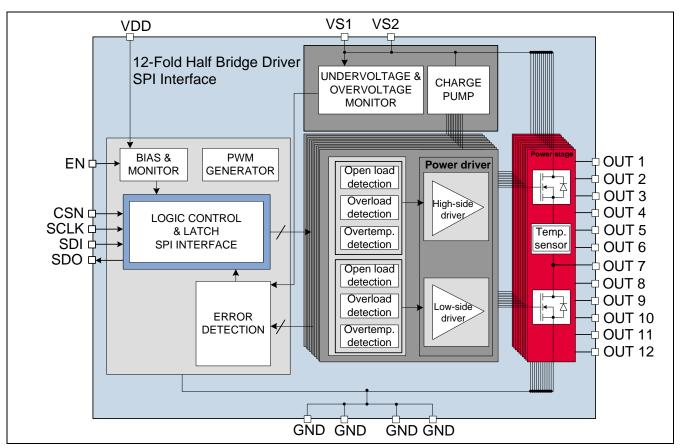
Figure 12 Block diagram TLE94112EL
