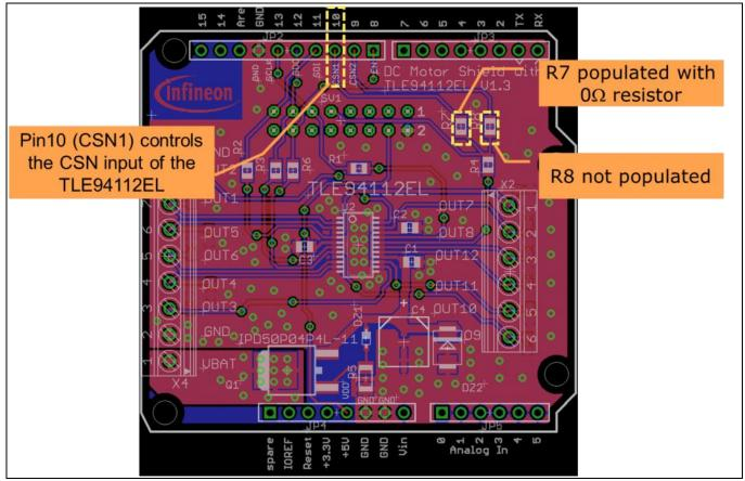
Figure 4 Figure 8 Control of CSN of TLE94112EL by Pin 10 (CSN1)
