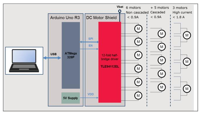
Figure 2 Simplified application diagram with TLE94112EL driving DC motors
