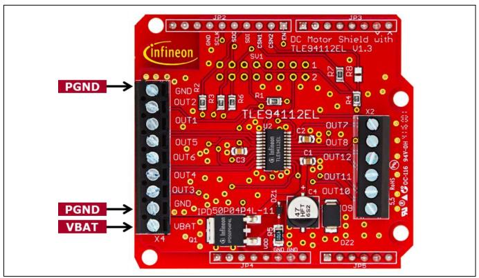
Figure 16 Supply connection
