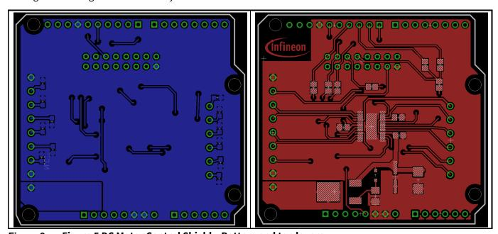
Figure 2 Figure 5 DC Motor Control Shield - Bottom and top layers
