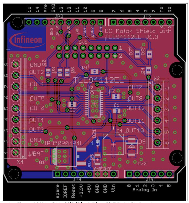
Figure 3 Figure 6 DC Motor Control Shield for Arduino with TLE94112EL - Layout
