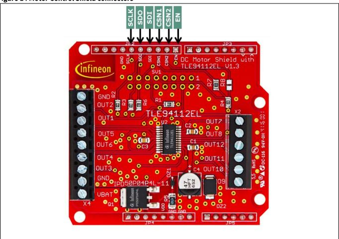
Figure 15 Control signals between DC motor shield and Arduino Uno
