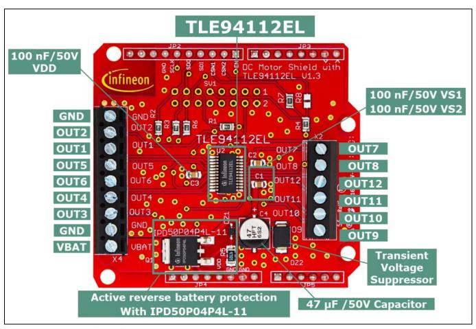
Figure 1 DC Motor Shield with TLE94112EL
