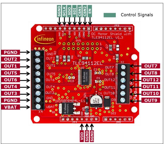
**Figure 3 DC Motor Control Shield connectors**
