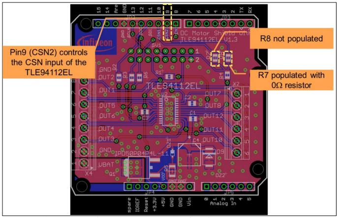
Figure 5 Figure 9 Control of CSN of TLE94112EL by Pin 9 (CSN2)
