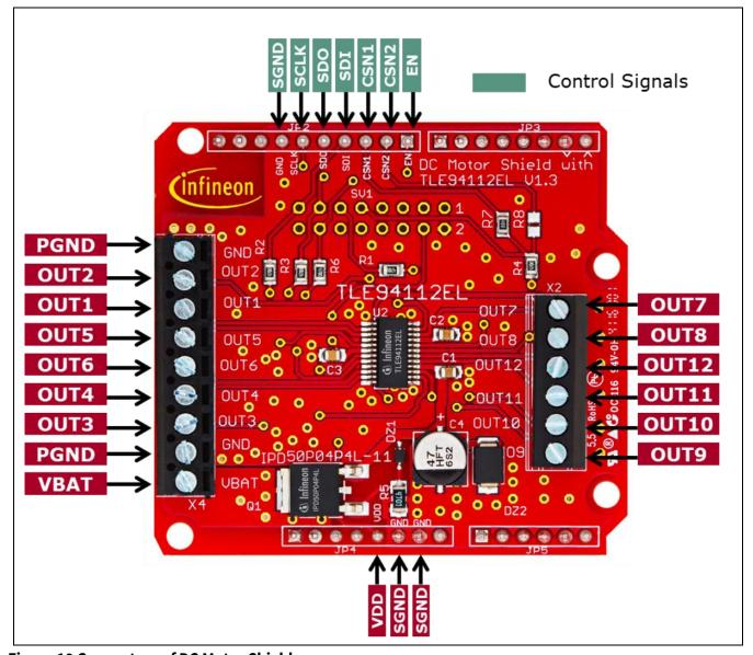
Figure 10 Connectors of DC Motor Shield
