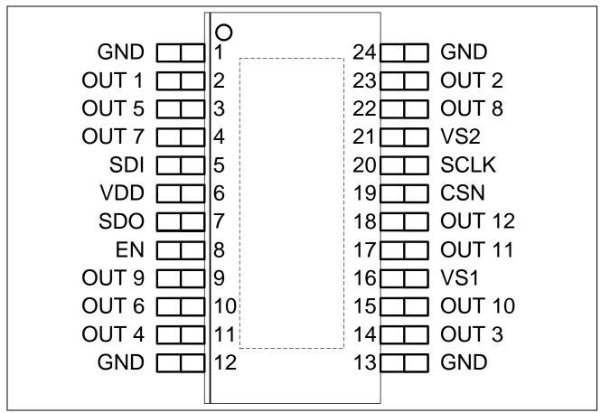
Figure 13 Pin assignment TLE94112EL (top view)
