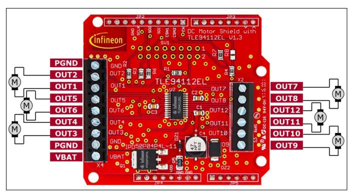
**Figure 14 Motor Control Shield connectors**
