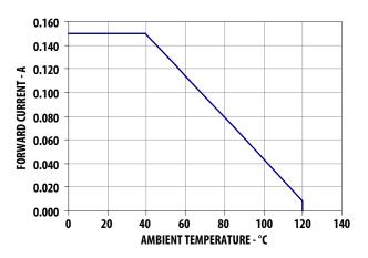
Figure 11: Maximum Pulse Current vs. Ambient Temperature  $T_{\text{A}}$  = 85° C
