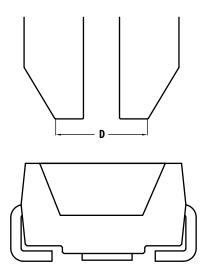
Note: Diameter "D" should be smaller than 2.2 mm SMT LED Indicator Components
