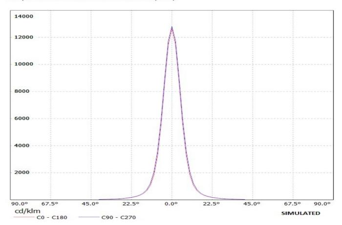
Luminaire: Ledil Oy FA10300\_OSS-D FA10300\_OSS-D Lamps: 1 x OSRAM-OS GOLDEN DRAGON+ (white)
