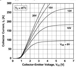
Figure 3. Typical Saturation Voltage Characteristics
