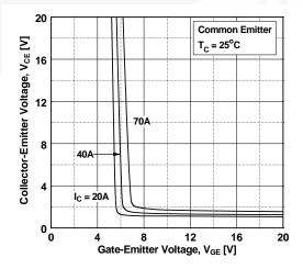
Figure 7. Saturation Voltage vs. V<sub>GE</sub>
