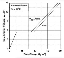
Figure 11. Turn-on Characteristics vs.
