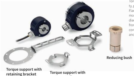
Torque supports offer a high degree of rotatory stability, preventing the encoder rotating along with the shaft. Flange adapters are used to mount the encoder on a motor. The reducing bushes allow you to reduce the diameter of a hollow shaft encoder. The encoder cables from PUR with M23 connector (encoder side) and open core (controller side) offer high flexibility, ruggedness and durability.
