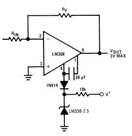
Figure 22. Op Amp with Output Clamped
