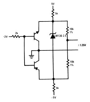
Figure 23. Bipolar Output Reference
