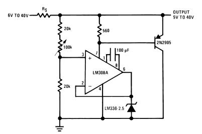
Figure 20. Adjustable Shunt Regulator
