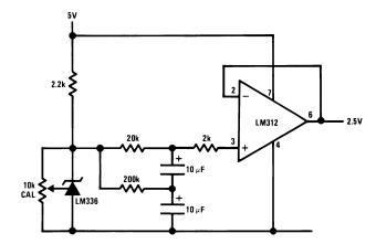
Figure 26. Low Noise Buffered Reference
