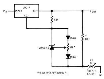
Figure 17. Precision Power Regulator with Low Temperature Coefficient
