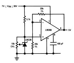
Figure 25. 5V Buffered Reference
