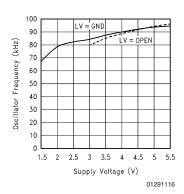
Oscillator Frequency vs Supply Voltage (FC = Open)
