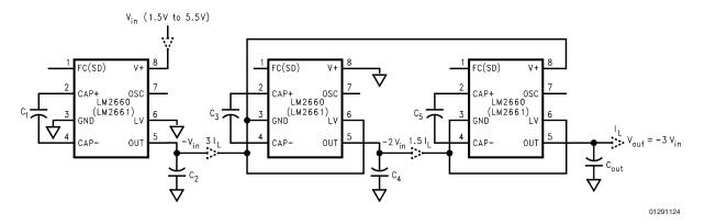
FIGURE 6. Generating -3V<sub>in</sub> from +V<sub>in</sub>
