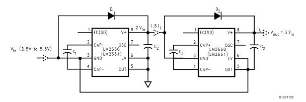
FIGURE 7. Generating +3V<sub>in</sub> from +V<sub>in</sub>
