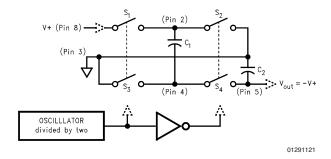
FIGURE 2. Voltage Inverting Principle
