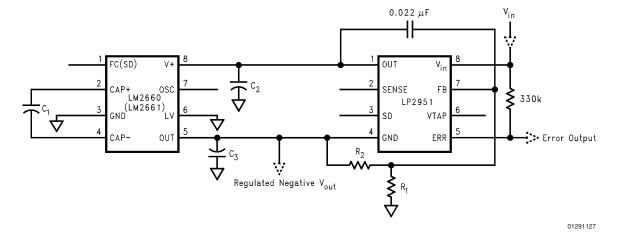
FIGURE 8. Combining LM2660/LM2661 with LP2951 to Make a Negative Adjustable Regulator
