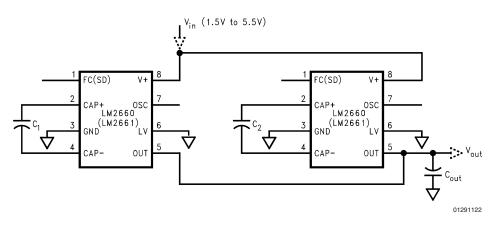
FIGURE 4. Lowering Output Resistance by Paralleling Devices
