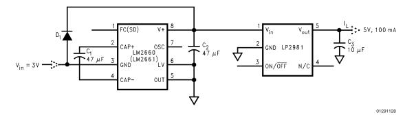
FIGURE 9. Generating +5V from +3V Input Voltage
