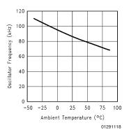
Oscillator Frequency vs Temperature (FC = Open)
