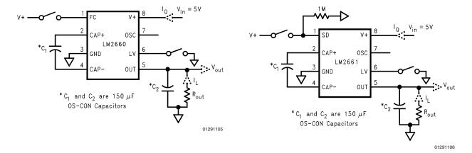
FIGURE 1. LM2660 and LM2661 Test Circuits
