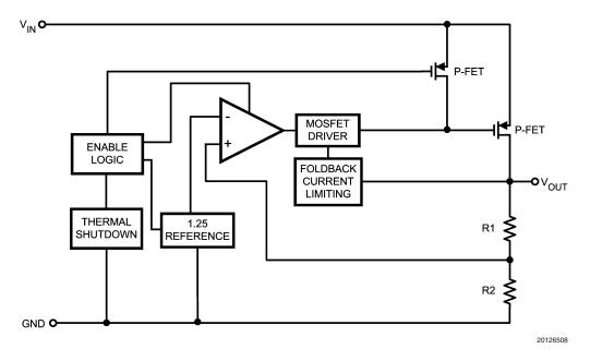
FIGURE 2. LP38691 Functional Diagram (TO-252)
