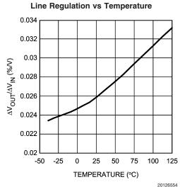
$\begin{tabular}{ll} \textbf{Typical Performance Characteristics} & \textbf{Unless otherwise specified:} & \textbf{T}_{J} = 25 ^{\circ} \textbf{C}, & \textbf{C}_{IN} = \textbf{C}_{OUT} = 10 \ \mu \textbf{F}, \\ \textbf{enable pin is tied to } & \textbf{V}_{IN} & \textbf{(LP38693 only)}, & \textbf{V}_{OUT} = 1.8 \mbox{V}, & \textbf{V}_{IN} = \mbox{V}_{OUT} + 1 \mbox{V}, & \textbf{I}_{L} = 10 \mbox{mA}. \\ \end{tabular}$
