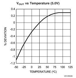
**Typical Performance Characteristics** Unless otherwise specified:  $T_J = 25^{\circ}C$ ,  $C_{IN} = C_{OUT} = 10~\mu\text{F}$ , enable pin is tied to  $V_{IN}$  (LP38693 only),  $V_{OUT} = 1.8V$ ,  $V_{IN} = V_{OUT} + 1V$ ,  $I_L = 10\text{mA}$ . (Continued)
