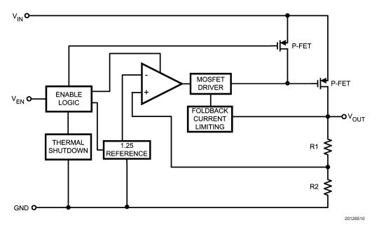
FIGURE 4. LP38693 Functional Diagram (SOT-223)
