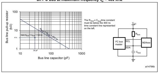
Figure 12. Maximum  $R_{bus}$  value versus bus parasitic capacitance ( $C_{bus}$ ) for an I<sup>2</sup>C bus at maximum frequency f<sub>C</sub> = 400 kHz
