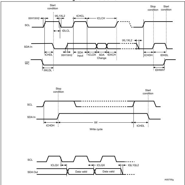
Figure 14. AC waveforms
