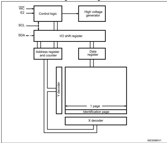
Figure 5. Block diagram
