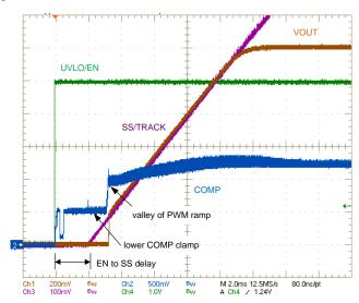
Figure 35. Typical Monotonic Output Voltage Startup Waveforms, 1.2-V Output
