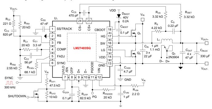
Figure 41. Application Circuit 1 with  $V_{IN}$  = 6.5 V to 20 V ( $V_{IN(nom)}$  = 12 V),  $V_{OUT}$  = 0.6 V to 5.3 V,  $I_{OUT(max)}$  = 25 A,  $F_{SW}$  = 300 kHz (Using External Synchronization Signal)
