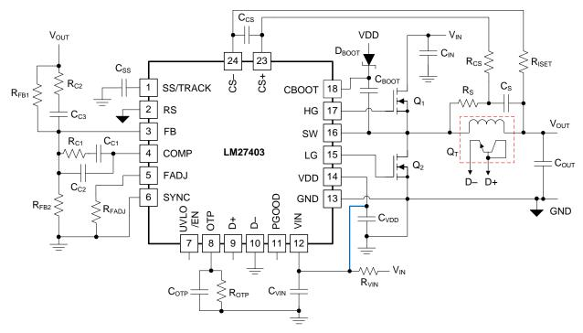
Figure 24. Schematic Diagram for VIN Operating Range of 3.0 V to 5.5 V
