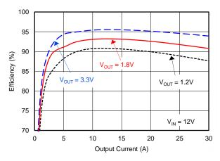
Figure 47. Efficiency vs. Output Current at  $V_{IN} = 12 \text{ V}$
