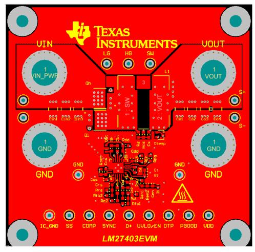
Figure 52. LM27403 PCB Layout
