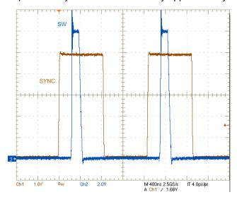
Figure 28. Typical 600-kHz SYNC Waveform
