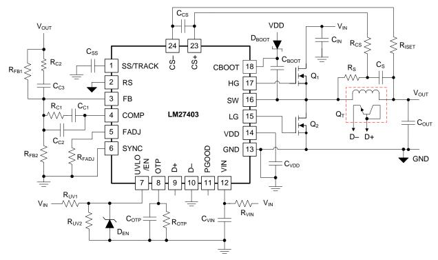
Figure 23. Schematic Diagram for VIN Operating Range of 3 V to 20 V
