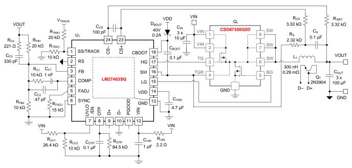
Figure 46. Application Circuit 2 With  $V_{IN} = 4.5 \text{ V}$  to 15 V ( $V_{IN(nom)} = 12 \text{ V}$ ),  $V_{OUT} = 1.8 \text{ V}$ ,  $I_{OUT(max)} = 30 \text{ A}$ ,  $F_{SW} = 600 \text{ kHz}$
