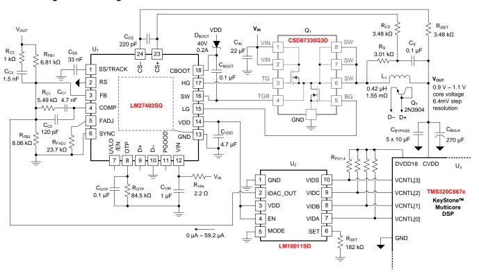
Figure 48. Application Circuit 3 with  $V_{IN} = 3 \text{ V}$  to 20 V,  $V_{OUT} = 0.9 \text{ V}$  to 1.1 V,  $I_{OUT(max)} = 15 \text{ A}$ ,  $F_{SW} = 450 \text{ kHz}$
