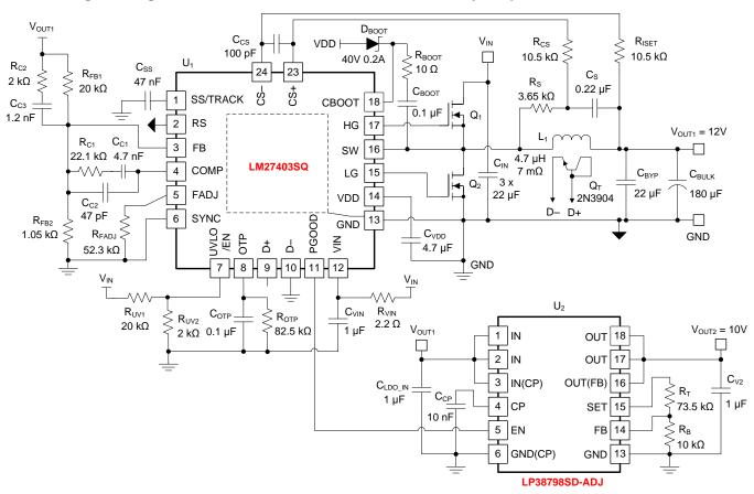
Figure 49. Application Circuit 4 with  $V_{IN}$  = 13 V to 20 V ( $V_{IN(nom)}$  = 18 V),  $V_{OUT1}$  = 12 V,  $I_{OUT1(max)}$  = 10 A,  $F_{SW}$  = 280 kHz,  $V_{OUT2}$  = 10 V,  $I_{OUT2(max)}$  = 0.8 A
