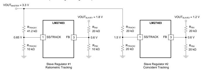
Figure 34. Tracking Implementation With Master, Ratiometric Slave and Coincident Slave Rails
