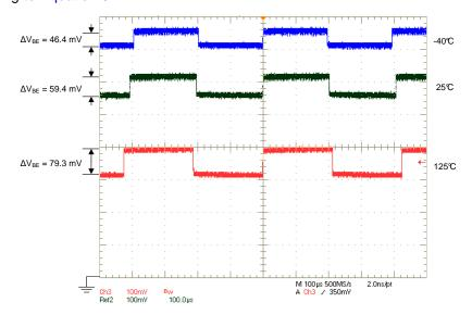
Figure 29. Typical 2N3904 Base-Emitter Voltage at -40°C, 25°C and 125°C
