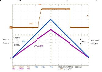
Figure 27. Typical Input Voltage UVLO Turn On and Off Behavior
