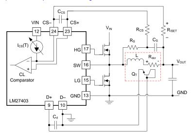
Figure 32. Current-Limit Setpoint Defined by Current Source I<sub>CS</sub> and Resistor R<sub>ISET</sub>
