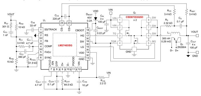
Figure 50. Application Circuit 5 With  $V_{IN}$  = 3.3 V to 5.5 V,  $V_{OUT}$  = 1 V,  $I_{OUT(max)}$  = 25 A,  $F_{SW}$  = 250 kHz
