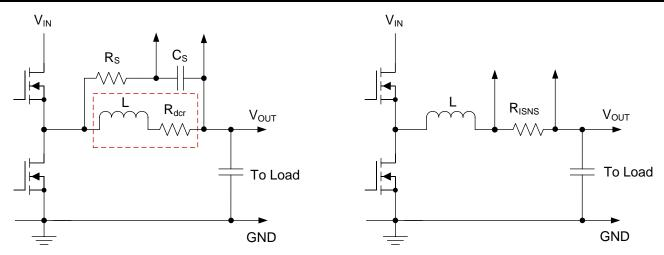
Figure 30. Current Sensing Using Inductor DCR
