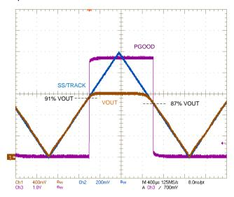
Figure 33. Typical Output Voltage Tracking Waveforms and PGOOD Flag
