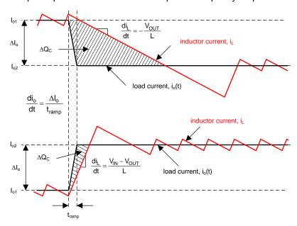
Figure 38. Load Transient Response Representation Showing Cour Charge Surplus Or Deficit.
