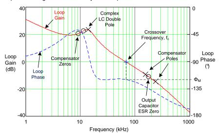
Figure 39. Typical Buck Regulator Loop Gain and Phase With Voltage-Mode Control
