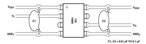
Figure 13. Recommended Printed Circuit Board Layout.
