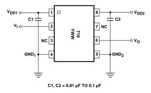
Figure 12. Recommended Printed Circuit Board Layout.
