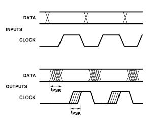
Figure 16. Parallel Data Transmission Example.
