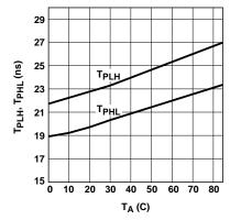
Figure 3. Typical Propagation Delays vs. Temperature.
