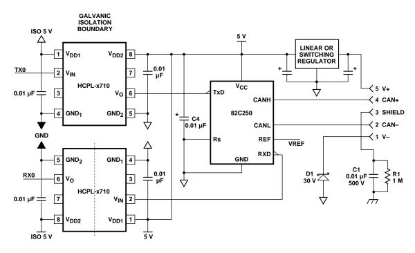
Figure 22. Recommended DeviceNet Application Circuit.
