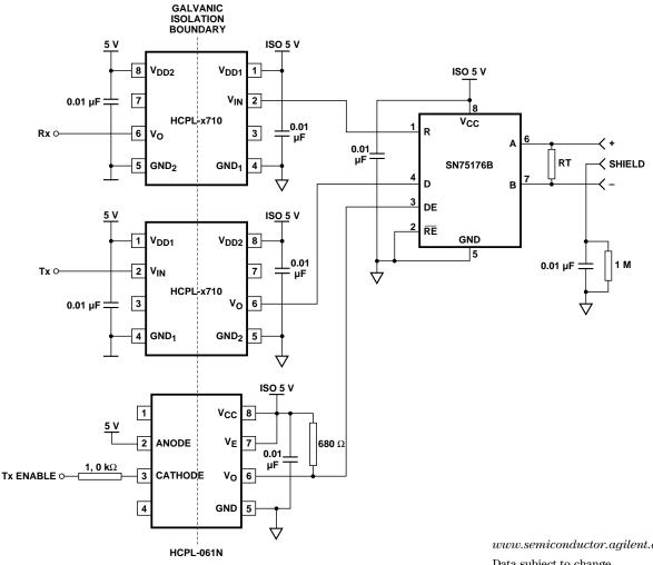
Figure 24. Recommended PROFIBUS Application Circuit.
