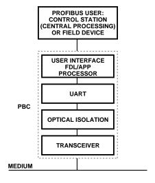
Figure 23. PROFIBUS Controller (PBC).
