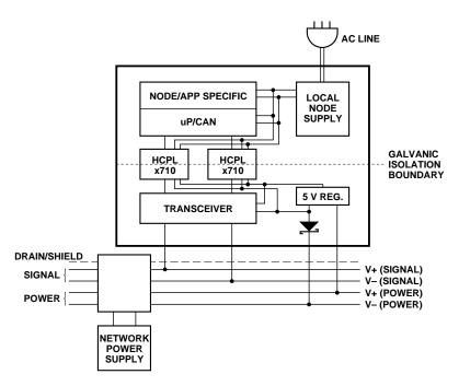
Figure 18. Typical DeviceNet Node.
