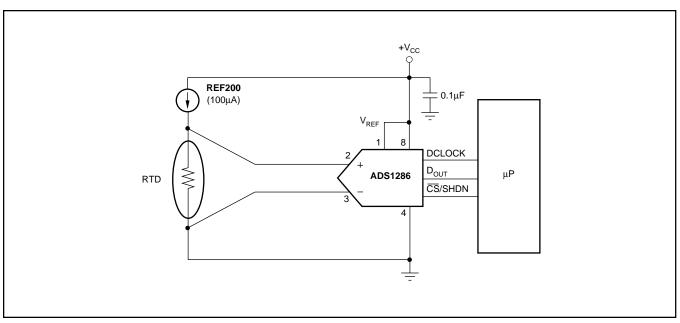
FIGURE 6. ADS1286 with RTD Sensor.
