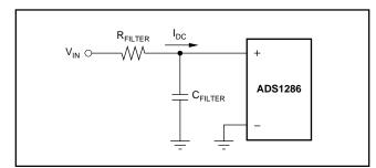
FIGURE 4. RC Input Filtering.
