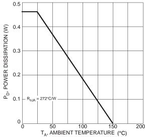
Fig. 3 Power Dissipation vs. Ambient Temperature
