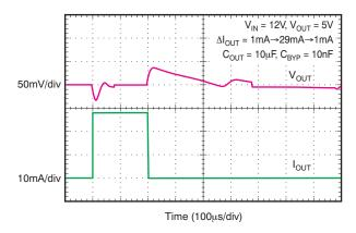
Figure 14. Load Transient Response
