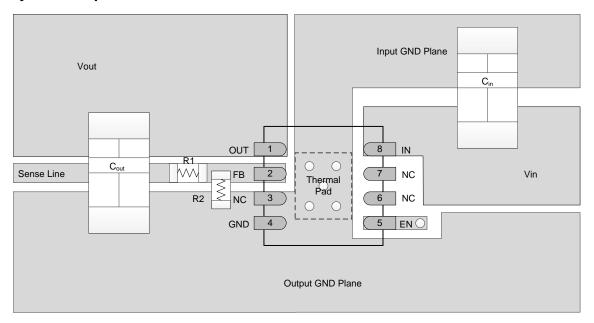
Figure 15. Recommended Layout Example
