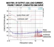
Measured on the MAX17501FTEVKIT with input filter—  $C_{IN}$  = 2.2 $\mu$ F,  $L_{IN}$  = 4.7 $\mu$ H, 2.2 $\mu$ F additional input capacitor used.
