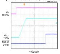
NO-LOAD SOFT-START FROM VIN (MAX17501B), 5V OUTPUT, FIGURE 7 CIRCUIT
