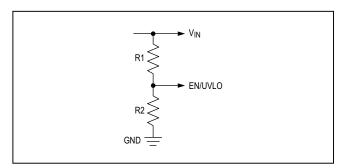
Figure 2. Adjustable EN/UVLO Network
