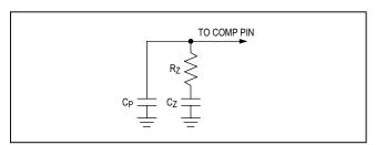
Figure 3. External Compensation Network
