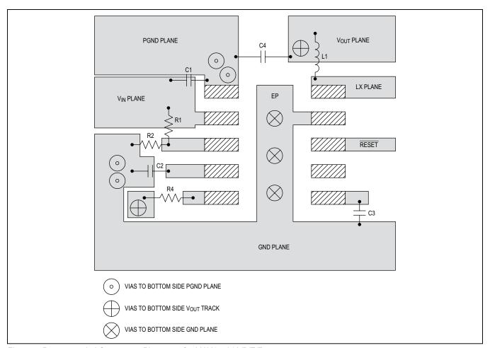
Figure 4. Recommended Component Placement for MAX17501A/B/E/F
