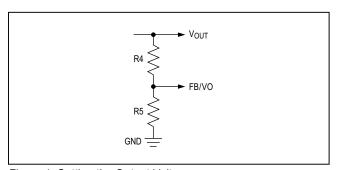
Figure 1. Setting the Output Voltage
