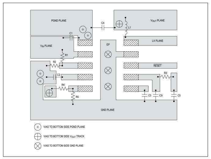
Figure 5. Recommended Component Placement for MAX17501G/H
