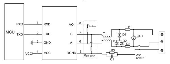
Fig. 2: Port protection circuit for harsh environments
