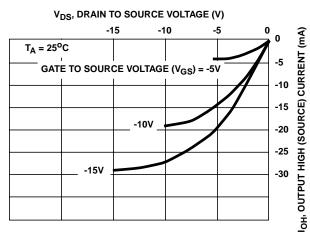
FIGURE 5. TYPICAL OUTPUT HIGH (SOURCE) CURRENT CHARACTERISTICS
