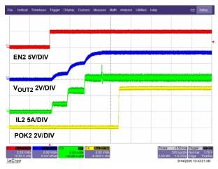
FIGURE 40. START-UP V<sub>OUT1</sub> = 3.3V (FULL LOAD, PWM MODE)
