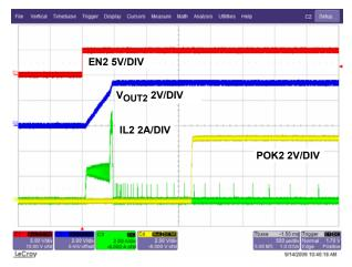
FIGURE 38. START-UP V<sub>OUT2</sub> = 3.3V (NO LOAD, SKIP MODE)
