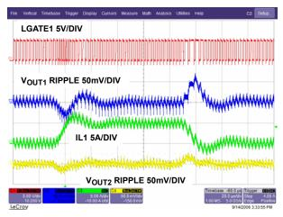
FIGURE 44. LOAD TRANSIENT V<sub>OUT1</sub> = 5V
