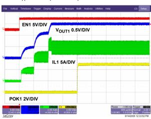
FIGURE 51. START-UP V<sub>OUT1</sub> = 1.5V (FULL LOAD, PWM MODE)
