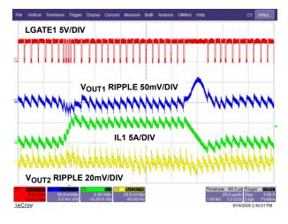
FIGURE 58. LOAD TRANSIENT V<sub>OUT1</sub> = 1.5V (PWM)
