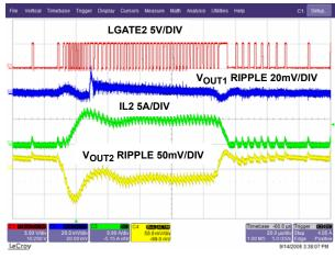
FIGURE 47. LOAD TRANSIENT V<sub>OUT1</sub> = 3.3V (SKIP)
