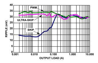
FIGURE 28. V<sub>OUT1</sub> = 5V RIPPLE vs LOAD
