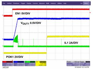
FIGURE 49. START-UP V<sub>OUT1</sub> = 1.5V (NO LOAD, SKIP MODE)
