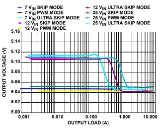
FIGURE 8. V<sub>OUT1</sub> = 5V REGULATION vs LOAD (400kHz)
