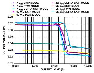
FIGURE 7. V<sub>OUT2</sub> = 3.3V REGULATION vs LOAD (500kHz)
