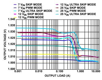
FIGURE 6. V<sub>OUT1</sub> = 1.5V REGULATION vs LOAD (200kHz)
