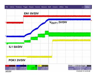
FIGURE 37. START-UP V<sub>OUT1</sub> = 5V (FULL LOAD, PWM MODE)
