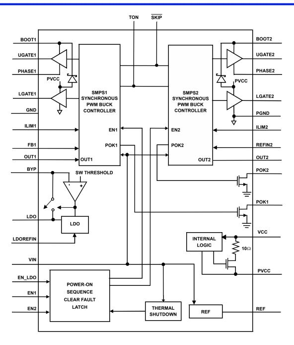
FIGURE 65. DETAILED FUNCTIONAL DIAGRAM ISL6237
