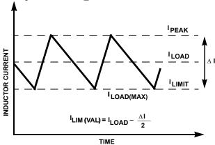
FIGURE 69. "VALLEY" CURRENT LIMIT THRESHOLD POINT
