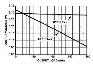
FIGURE 30. LDO OUTPUT 3.3V vs LOAD
