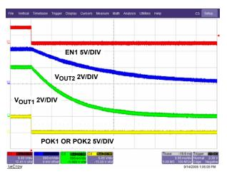
FIGURE 57. SHUTDOWN ( $V_{OUT1} = 1.5V$ ,  $V_{OUT2} = 1.05V$ , EN2 = REF)
