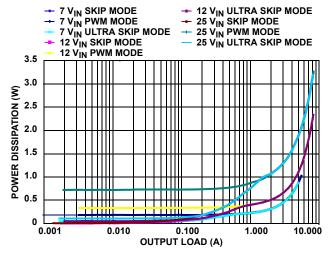
FIGURE 12. V<sub>OUT1</sub> = 5V POWER DISSIPATION vs LOAD (400kHz)
