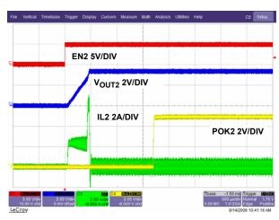
FIGURE 39. START-UP V<sub>OUT1</sub> = 3.3V (NO LOAD, PWM MODE)
