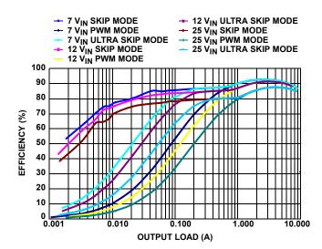
FIGURE 2. V<sub>OUT1</sub> = 1.5V EFFICIENCY vs LOAD (200kHz)
