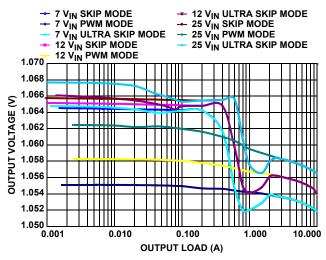
FIGURE 5. V<sub>OUT2</sub> = 1.05V REGULATION vs LOAD (300kHz)
