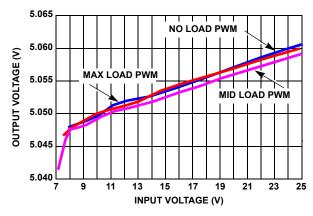
FIGURE 19.  $V_{OUT1}$  = 5V OUTPUT VOLTAGE REGULATION vs  $V_{IN}$  (PWM MODE)
