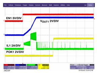
FIGURE 35. START-UP V<sub>OUT1</sub> = 5V (NO LOAD, SKIP MODE)
