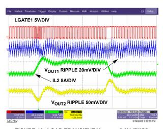
FIGURE 46. LOAD TRANSIENT V<sub>OUT1</sub> = 3.3V (PWM)
