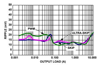
FIGURE 22. V<sub>OUT2</sub> = 1.05V RIPPLE vs LOAD
