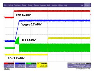
FIGURE 50. START-UP  $V_{OUT1}$  = 1.5V (NO LOAD, PWM MODE)S
