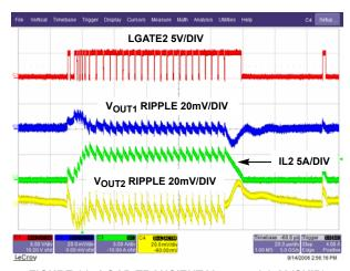
FIGURE 61. LOAD TRANSIENT V<sub>OUT1</sub> = 1.05V (SKIP)
