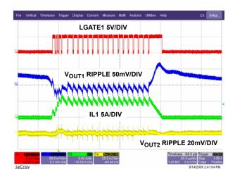
FIGURE 59. LOAD TRANSIENT V<sub>OUT1</sub> = 1.5V (SKIP)
