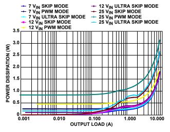
FIGURE 11. V<sub>OUT2</sub> = 3.3V POWER DISSIPATION vs LOAD (500kHz)
