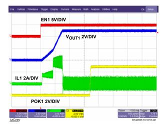
FIGURE 36. START-UP V<sub>OUT1</sub> = 5V (NO LOAD, PWM MODE)
