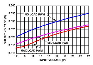
FIGURE 17.  $V_{OUT2}$  = 3.3V OUTPUT VOLTAGE REGULATION vs  $V_{IN}$  (PWM MODE)
