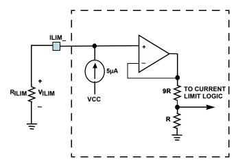
FIGURE 70. CURRENT LIMIT BLOCK DIAGRAM
