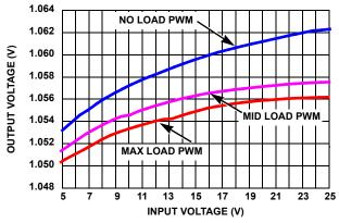
FIGURE 13.  $V_{OUT2}$  = 1.05V OUTPUT VOLTAGE REGULATION vs  $V_{IN}$  (PWM MODE)
