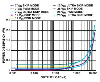
FIGURE 10. V<sub>OUT1</sub> = 1.5V POWER DISSIPATION vs LOAD (200kHz)
