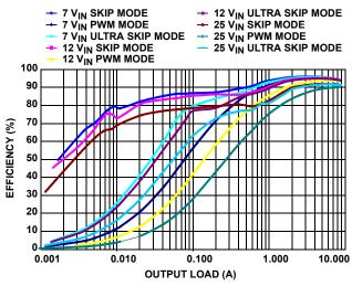
FIGURE 3. V<sub>OUT2</sub> = 3.3V EFFICIENCY vs LOAD (500kHz)
