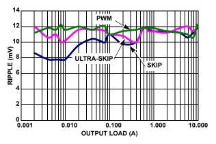
FIGURE 26. V<sub>OUT2</sub> = 3.3V RIPPLE vs LOAD
