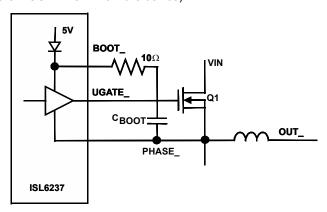
FIGURE 71. REDUCING THE SWITCHING-NODE RISE TIME
