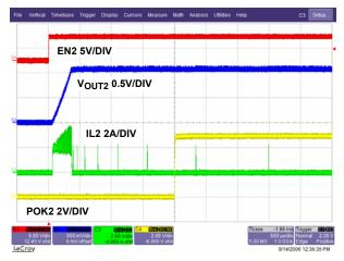
FIGURE 52. START-UP  $V_{OUT2} = 1.05V$  (NO LOAD, SKIP MODE)
