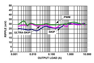
FIGURE 24. V<sub>OUT1</sub> = 1.5V RIPPLE vs LOAD
