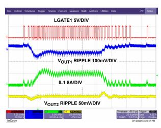
FIGURE 45. LOAD TRANSIENT V<sub>OUT1</sub> = 5V (SKIP)
