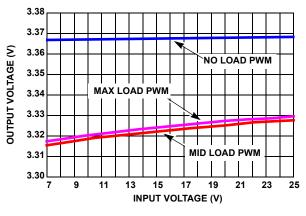
FIGURE 18.  $V_{OUT2}$  = 3.3V OUTPUT VOLTAGE REGULATION vs  $V_{IN}$  (SKIP MODE)
