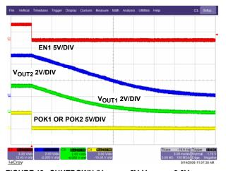
FIGURE 43. SHUTDOWN ( $V_{OUT1}$  = 5V,  $V_{OUT2}$  = 3.3V, EN2 = REF)
