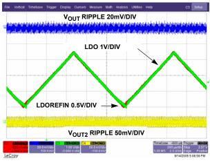
FIGURE 48. LDO TRACKING TO LDOREFIN
