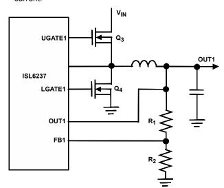
FIGURE 72. SETTING V<sub>OUT1</sub> WITH A RESISTOR DIVIDER
