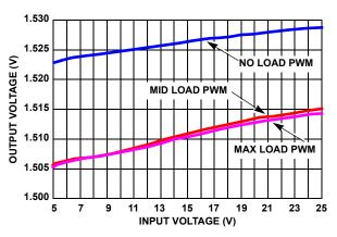
FIGURE 16.  $V_{OUT1}$  = 1.5V OUTPUT VOLTAGE REGULATION vs  $V_{IN}$  (SKIP MODE)
