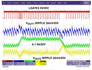
FIGURE 60. LOAD TRANSIENT V<sub>OUT1</sub> = 1.05V (PWM)
