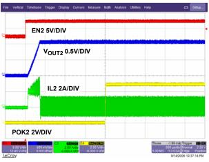
FIGURE 53. START-UP  $V_{OUT1}$  = 1.05V (NO LOAD, PWM MODE)
