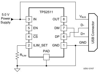
Figure 17. 5-W USB Charger Application Without Power Switch
