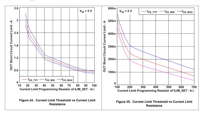
For this example design, as shown in Equation 8,  $I_{OS MIN} = 2100$  mA.
