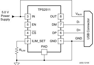
Figure 15. 10-W USB Charger Application Without Power Switch
