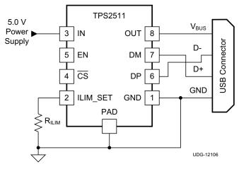
Figure 16. 5-W USB Charger Application With Power Switch
