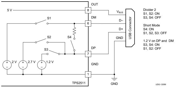
Figure 22. TPS2511 DCP Auto-Detect Functional Diagram
