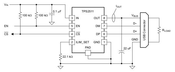
Figure 23. Test Circuit for System Operation
