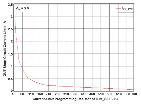
Figure 11. Typical Current Limit vs Programming Resistor
