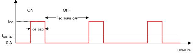
Figure 10. OUT Pin Short-Circuit Current in Hiccup Mode
