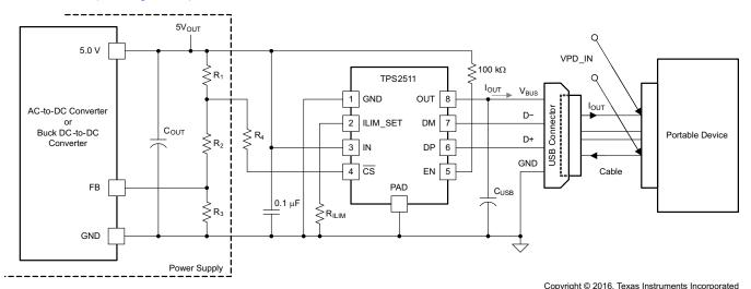
Figure 12. TPS2511 Charging System Schematic Diagram
