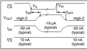
**FIGURE 1-1:** Timing Diagram for the  $\overline{\text{CS}}$  Pin on the MCP618.
