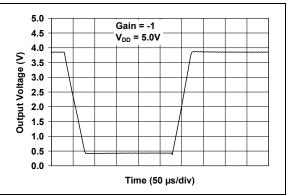
**FIGURE 2-34:** Large-Signal, Inverting Pulse Response.
