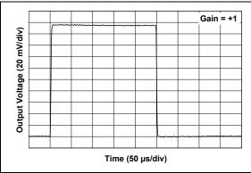
**FIGURE 2-27:** Small-Signal, Non-Inverting Pulse Response.
