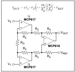
FIGURE 4-11: Three-Op Amp Instrumentation Amplifier.
