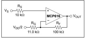
FIGURE 4-9: High Gain Pre-amplifier.
