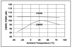
**FIGURE 2-11:** CMRR, PSRR vs. Ambient Temperature.
