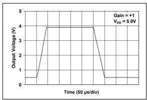
**FIGURE 2-31:** Large-Signal, Non-Inverting Pulse Response.
