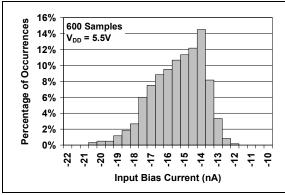
**FIGURE 2-3:** Input Bias Current at  $V_{DD} = 5.5V$ .
