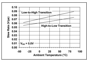
FIGURE 2-14: Slew Rate vs. Ambient Temperature.
