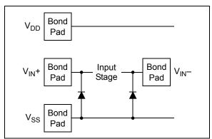
FIGURE 4-1: Simplified Analog Input ESD Structures.
