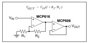
FIGURE 4-12: Precision Gain with Good Load Isolation.
