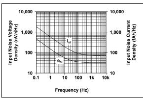
**FIGURE 2-26:** Input Noise Voltage, Current Densities vs. Frequency.
