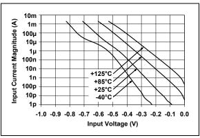
**FIGURE 2-36:** Measured Input Current vs. Input Voltage (below  $V_{SS}$ ).
