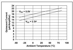
**FIGURE 2-8:** Quiescent Current vs. Ambient Temperature.
