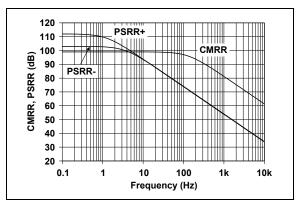
**FIGURE 2-28:** CMRR, PSRR vs. Frequency.
