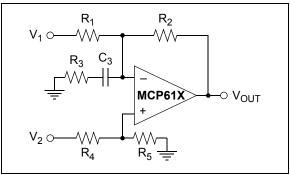
FIGURE 4-3: Example Circuit for Calculating DC Offset.
