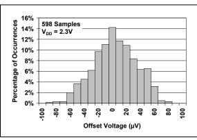
FIGURE 2-2: Input Offset Voltage at  $V_{DD} = 2.3V$ .
