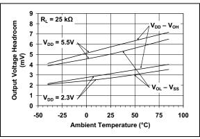
**FIGURE 2-12:** Maximum Output Voltage Swing vs. Ambient Temperature at  $R_L = 25 \text{ k}\Omega$ .
