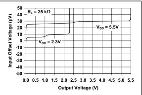
FIGURE 2-18: Input Offset Voltage vs. Output Voltage.
