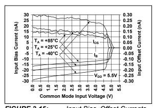
**FIGURE 2-15:** Input Bias, Offset Currents vs. Common-mode Input Voltage.
