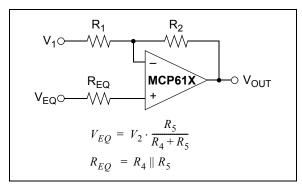
FIGURE 4-4: Equivalent DC Circuit.
