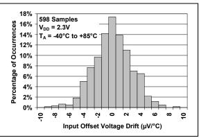
FIGURE 2-5: Input Offset Voltage Drift at  $V_{DD} = 2.3V$ .
