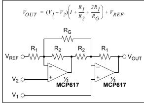
FIGURE 4-10: Two-Op Amp Instrumentation Amplifier.
