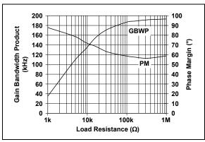
**FIGURE 2-21:** Gain-Bandwidth Product, Phase Margin vs. Load Resistance.
