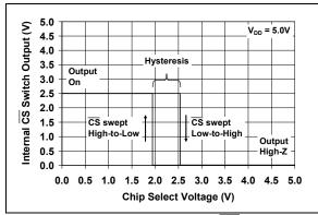
**FIGURE 2-35:** Chip Select  $(\overline{CS})$  Internal Hysteresis (MCP618 only).
