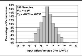
FIGURE 2-4: Input Offset Voltage Drift at  $V_{DD} = 5.5V$ .
