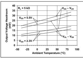
**FIGURE 2-9:** Maximum Output Voltage Swing vs. Ambient Temperature at  $R_L = 5 \text{ k}\Omega$ .
