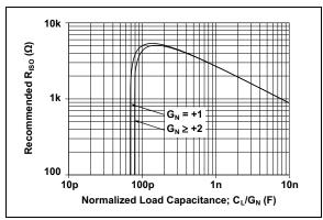
**FIGURE 4-6:** Recommended R<sub>ISO</sub> Values for Capacitive Loads.
