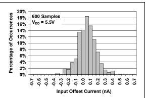
FIGURE 2-6: Input Offset Current at  $V_{DD} = 5.5V$ .
