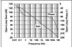
FIGURE 2-25: Open-Loop Gain, Phase vs. Frequency.
