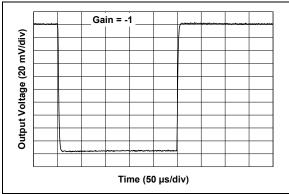
FIGURE 2-30: Small-Signal, Inverting Pulse Response.
