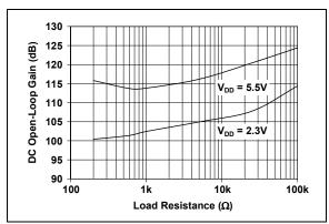
**FIGURE 2-20:** DC Open-Loop Gain vs. Load Resistance.
