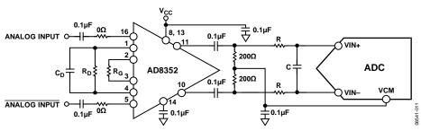
Figure 41. Differential Input Configuration Using the AD8352
