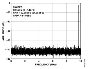
Figure 24. AD9609-20 Single-Tone FFT with  $f_{\text{IN}}$  = 30.5 MHz
