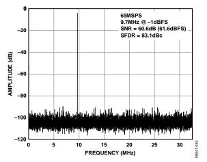
Figure 15. AD9609-65 Single-Tone FFT with  $f_{\text{IN}} = 9.7 \text{ MHz}$
