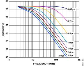
Figure 52. SNR vs. Input Frequency and Jitter
