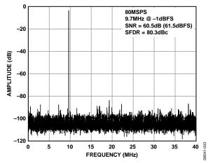
Figure 4. AD9609-80 Single-Tone FFT with  $f_{IN} = 9.7$  MHz
