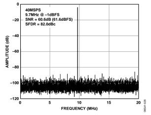
Figure 20. AD9609-40 Single-Tone FFT with  $f_{\text{IN}} = 9.7 \text{ MHz}$
