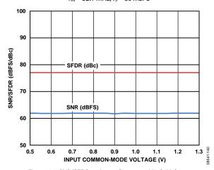
Figure 36. SNR/SFDR vs. Input Common-Mode Voltage,  $f_{IN} = 10.3$  MHz,  $f_{S} = 20$  MSPS
