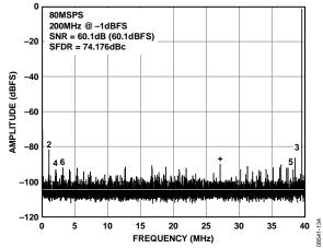
Figure 8. AD9609-80 Single-Tone FFT with  $f_{IN} = 200 \text{ MHz}$
