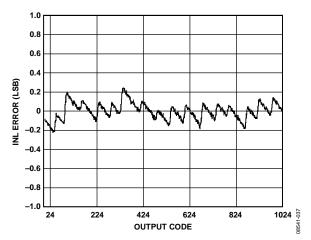
Figure 14. INL with  $f_{IN} = 9.7 \text{ MHz}$
