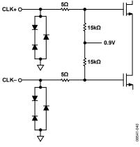
Figure 29. Equivalent Clock Input Circuit
