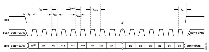
Figure 54. Serial Port Interface Timing Diagram
