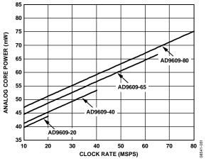
Figure 53. AD9609 Analog Core Power vs. Clock Rate
