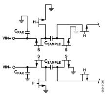
Figure 34. Switched-Capacitor Input Circuit
