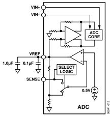
Figure 42. Internal Reference Configuration
