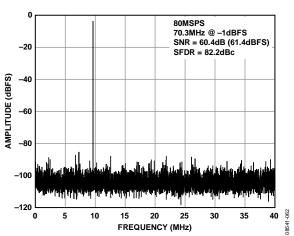
Figure 5. AD9609-80 Single-Tone FFT with  $f_{IN} = 70.3$  MHz
