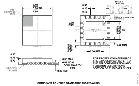
Figure 55. 32-Lead Lead Frame Chip Scale Package [LFCSP] 5 mm × 5 mm Body and 0.75 mm Package Height (CP-32-11) Dimensions shown in millimeters
