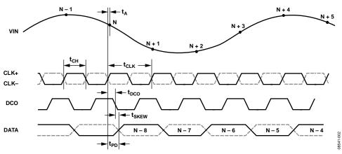
Figure 2. CMOS Output Data Timing
