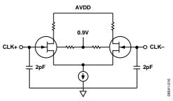
Figure 45. Equivalent Clock Input Circuit
