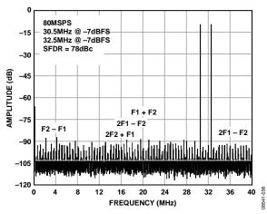
Figure 6. AD9609-80 Two-Tone FFT with  $f_{IN1} = 30.5$  MHz and  $f_{IN2} = 32.5$  MHz
