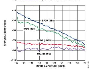
Figure 9. Two-Tone SFDR/IMD3 vs. Input Amplitude (AIN) with  $f_{\rm IN1}=30.5$  MHz and  $f_{\rm IN2}=32.5$  MHz
