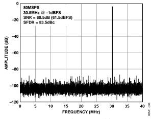
Figure 7. AD9609-80 Single-Tone FFT with  $f_{IN} = 30.5$  MHz
