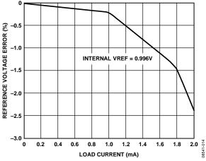
Figure 43. VREF Accuracy vs. Load Current
