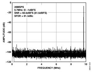
Figure 23. AD9609-20 Single-Tone FFT with  $f_{IN} = 9.7$  MHz
