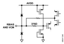
Figure 33. Equivalent RBIAS and VCM Circuit
