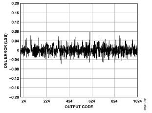
Figure 13. DNL Error with  $f_{IN} = 9.7 \text{ MHz}$
