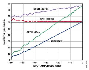
Figure 25. AD9609-20 SNR/SFDR vs. Input Amplitude (AIN) with  $f_{\rm IN}$  = 9.7 MHz
