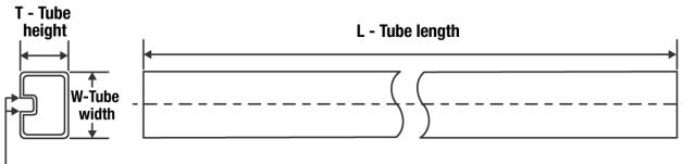
B - Alignment groove width
