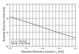
Figure 9. Reverse Recovery Time vs Reverse Recovery Current
