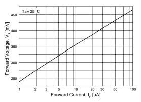
Figure 4. Forward Voltage vs Forward Current VF - 1.0 to 100uA
