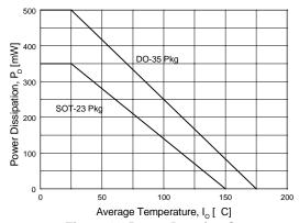
Figure 11. Power Derating Curve
