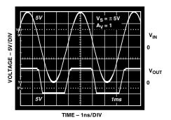
Figure 2. Output Voltage Phase Reversal Behavior
