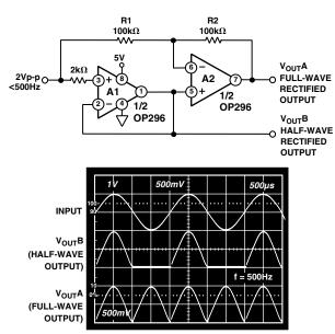
Figure 6. Single-Supply Half-Wave and Full-Wave Rectifiers Using an OP296
