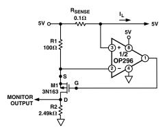
Figure 11. A High-Side Load Current Monitor
