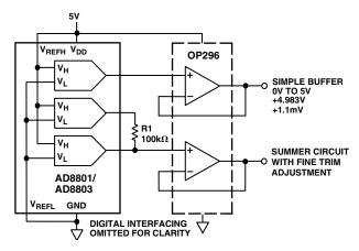
Figure 10. Buffering a TrimDAC OutputTPC
