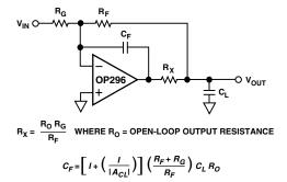
Figure 4. In-the-Loop Compensation Technique for Driving Capacitive Loads
