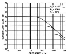
TPC 20. Closed-Loop Gain vs. Frequency
