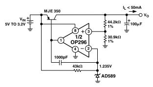
Figure 8. 3 V Low Dropout Voltage Regulator
