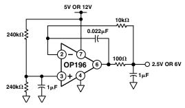
Figure 5. A Micropower False-Ground Generator
