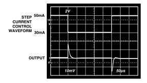
Figure 9. Output Step Load Current Recovery
