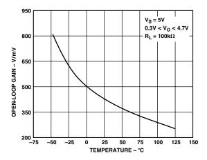
TPC 18. Open-Loop Gain vs. Temperature
