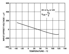
TPC 6. Input Offset Voltage vs. Temperature
