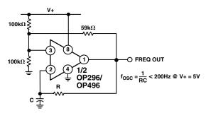
Figure 7. Square Wave Oscillator Has Stable Frequency Regardless of Supply Voltage Changes
