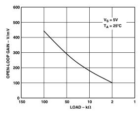
TPC 19. Open-Loop Gain vs. Resistive Load
