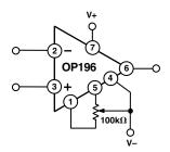
Figure 3. Offset Nulling Circuit
