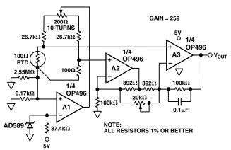
Figure 12. A Single-Supply RTD Amplifier
