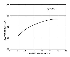
TPC 26. Supply Current/Amplifier vs. Supply Voltage
