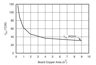
NOTE:  $\theta_{JA}$  value at a board size of 9-in<sup>2</sup> (that is, 3-in × 3-in) is a JEDEC standard.
