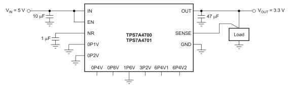
Figure 24. Typical Application, V<sub>OUT</sub> = 3.3 V
