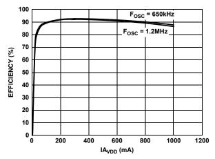
FIGURE 1.  $A_{VDD}$  EFFICIENCY vs  $IA_{VDD}$
