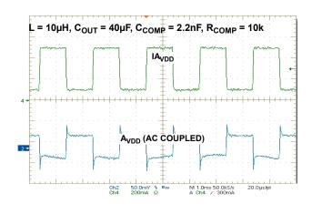
FIGURE 4. BOOST CONVERTER TRANSIENT RESPONSE
