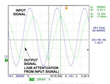
FIGURE 12.  $V_{COM}$  BANDWIDTH MEASUREMENT
