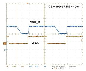
FIGURE 8. GPM CIRCUIT WAVEFORM
