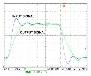
FIGURE 11.  $V_{\text{COM}}$  RISING SLEW RATE
