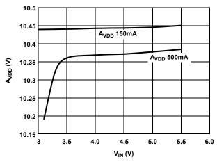
FIGURE 3. LINE REGULATION  $\mathbf{A}_{VDD}$  vs  $\mathbf{V}_{IN}$
