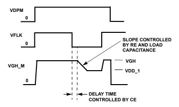
FIGURE 17. GATE PULSE MODULATOR TIMING DIAGRAM
