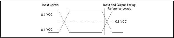
AC Measurement I/O Waveform
