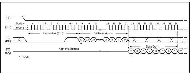
Figure 9. Read Data Instruction Sequence Diagram
