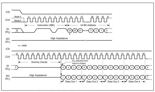
Figure 11. Fast Read Dual Output Instruction Sequence Diagram
