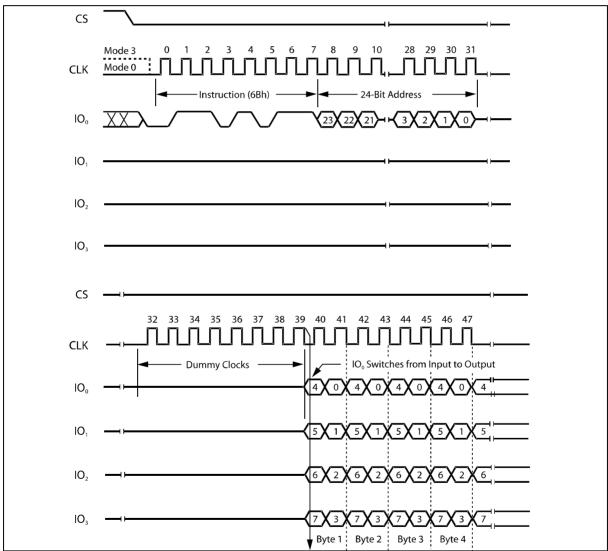
Figure 12. Fast Read Quad Output Instruction Sequence Diagram
