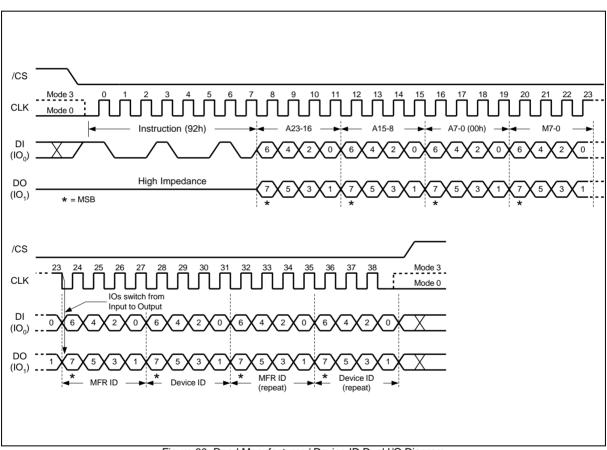
Figure 30. Read Manufacturer / Device ID Dual I/O Diagram
