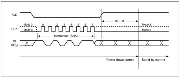
Figure 28a. Release Power-down Instruction Sequence
