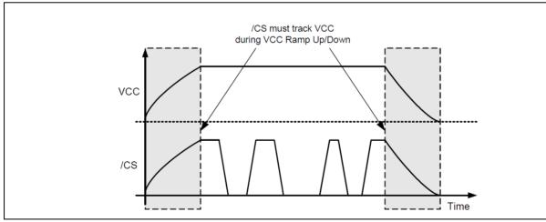
Figure 40b. Power-up, Power-Down Requirement
