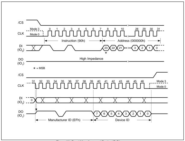
Figure 29. Read Manufacturer / Device ID Diagram
