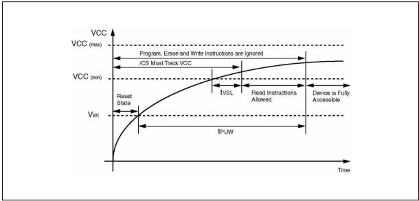
Figure 40a. Power-up Timing and Voltage Levels
