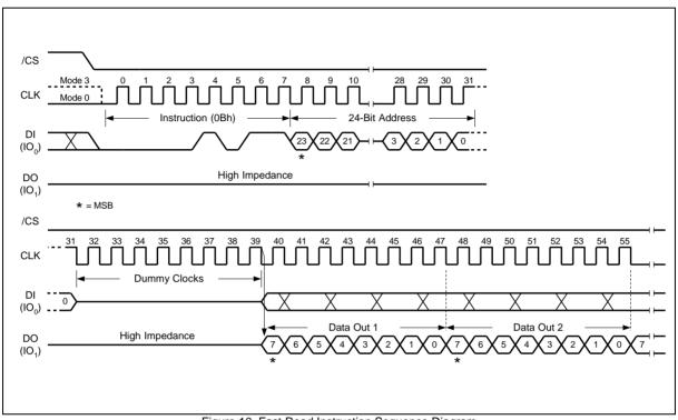
Figure 10. Fast Read Instruction Sequence Diagram
