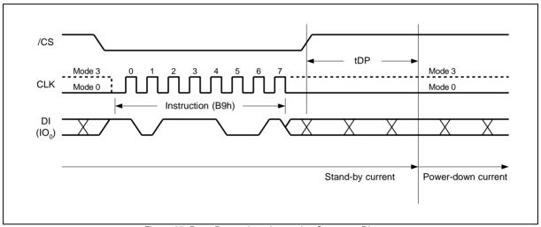
Figure 27. Deep Power-down Instruction Sequence Diagram
