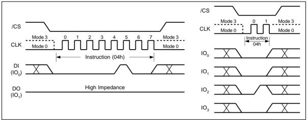
Figure 6. Write Disable Instruction Sequence Diagram
