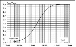
Figure 7. Non-repetitive peak surge forward current versus pulse duration (sinusoidal waveform, per diode)
