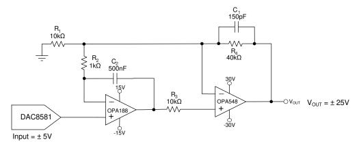
Figure 49. Programmable Power Supply
