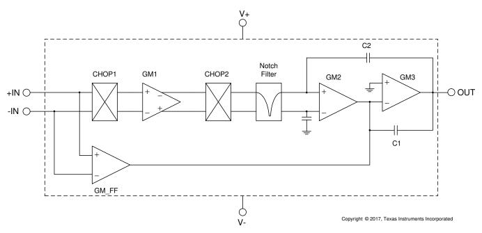
Figure 38. Functional Block Diagram
