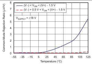
Figure 13. CMRR vs Temperature
