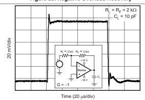
Figure 29. Small-Signal Step Response (100 mV)
