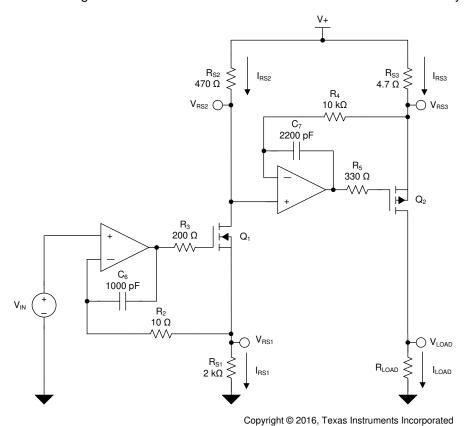
Figure 44. High-Side Voltage-to-Current (V-I) Converter
