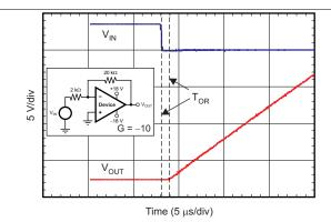
Figure 27. Positive Overload Recovery
