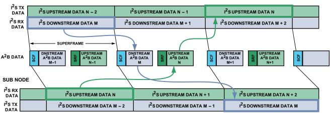
Figure 4. A<sup>2</sup>B Bus Synchronous Data Exchange
