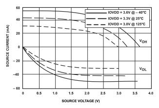
Figure 26. Digital I/O Drivers (DS1, 3.3 V IOVDD)
