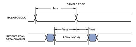
Figure 9. PDM Timing
