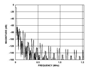
Figure 19. PDM Out of Band Frequency Response ( $f_{SYNCM} = 48 \text{ kHz}$ )
