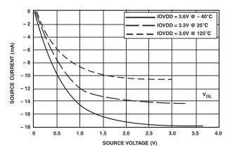
Figure 24. I<sup>2</sup>C Drivers (3.3 V IOVDD)
