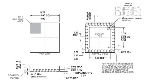
Figure 40. 32-Lead Lead Frame Chip Scale Package [LFCSP\_SS] 5 mm x 5 mm Body, With Side Solderable Leads (CS-32-3) Dimensions shown in millimeters
