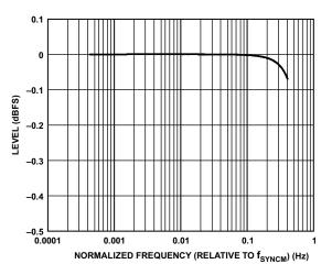
Figure 16. PDM Frequency Response,  $f_{SYNCM} = 48 \text{ kHz}$
