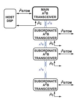
Figure 2. Communication System Block Diagram
