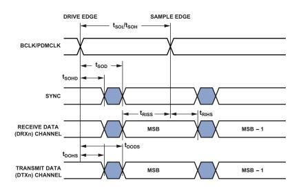
Figure 12. I<sup>2</sup>S Master (A<sup>2</sup>B Subordinate Node) Timing
