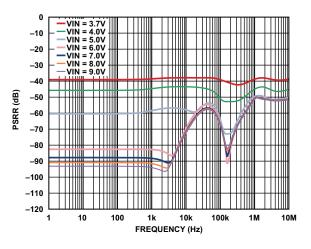
Figure 8. VOUT2 PSRR,  $I_{VOUT2} = 50 \text{ mA}$
