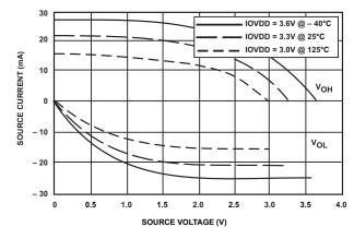
Figure 22. Digital I/O Drivers (DS0, 3.3 V IOVDD)
