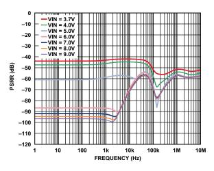
Figure 7. VOUT2 PSRR,  $I_{VOUT2} = 10 \text{ mA}$
