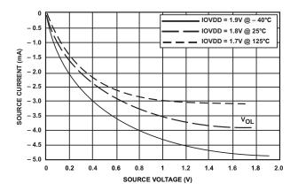
Figure 23. I<sup>2</sup>C Drivers (1.8 V IOVDD)
