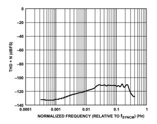
Figure 18. PDM Total Harmonic Distortion + Noise (THD + N) vs. Normalized Frequency (Relative to  $f_{SYNCM}$ ,  $f_{SYNCM} = 48$  kHz
