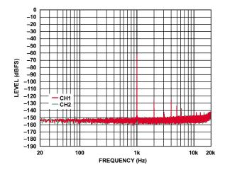
Figure 15. PDM FFT,  $f_{SYNCM} = 48 \text{ kHz}$ , -60 dBFS Input
