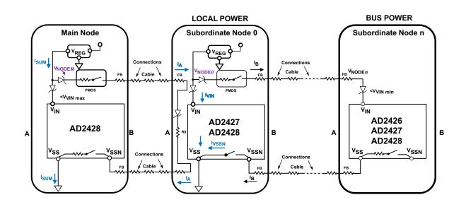
Figure 36. A<sup>2</sup>B DC Power Model for a System with Local and Bus Powered Subordinates
