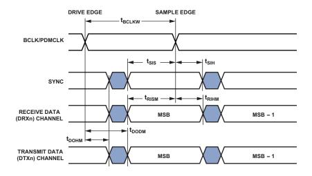
Figure 11. I<sup>2</sup>S Slave (A<sup>2</sup>B Main Node) Timing
