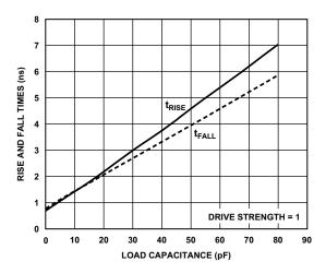
Figure 33. Digital I/O Driver Typical Rise and Fall Times (10% to 90%) vs. Load Capacitance (V<sub>IOVDD</sub> = 3.3 V, T<sub>J</sub> = 25°C)
