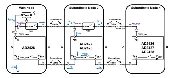
Figure 37. A<sup>2</sup>B Power Model for Bus Powered System
