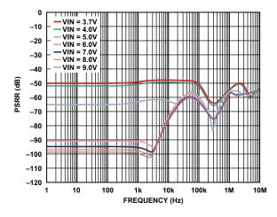
Figure 6. VOUT1 PSRR, I<sub>VOUT1</sub> = 40 mA
