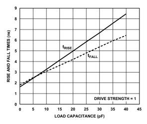
Figure 31. Digital I/O Driver Typical Rise and Fall Times (10% to 90%) vs. Load Capacitance ( $V_{IOVDD} = 1.8 V, T_J = 25^{\circ}C$ )
