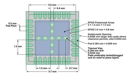
Figure 39. Transceiver Footprint
