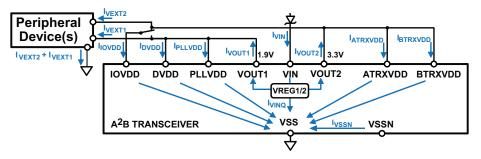
Figure 35. Current Flow Model
