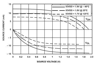
Figure 25. Digital I/O Drivers (DS1, 1.8 V IOVDD)
