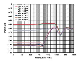
Figure 5. VOUT1 PSRR,  $I_{VOUT1} = 10 \text{ mA}$
