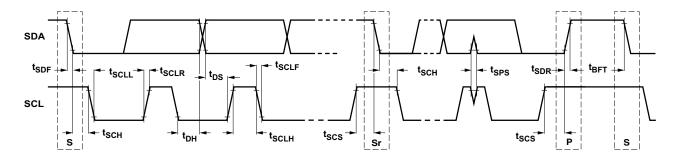
Figure 10. I<sup>2</sup>C Port Timing
