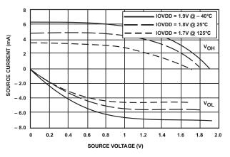
Figure 21. Digital I/O Drivers (DS0, 1.8 V IOVDD)
