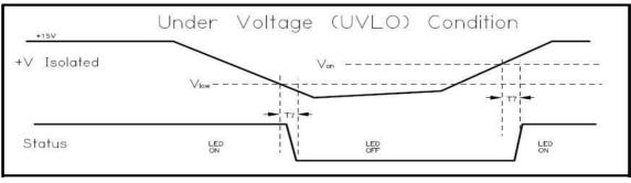
Figure 5: Signal fault timing diagram for UVLO.
