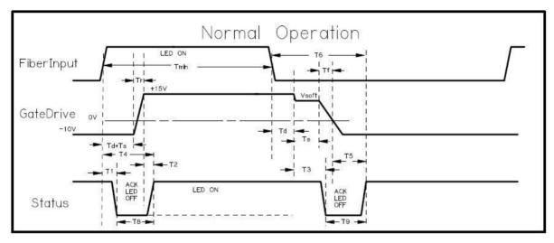
Figure 3: Signal input and output timing diagram
