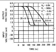
Figure 19. Response Time for Various Input Overdrives
