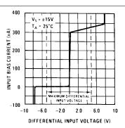
Figure 18. Input Characteristics
