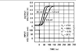
Figure 17. Response Time for Various Input Overdrives
