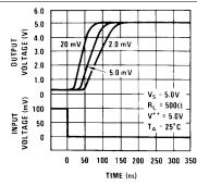
Figure 20. Response Time for Various Input Overdrives
