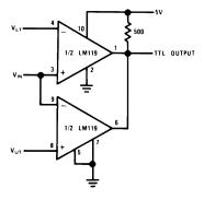
Figure 26. Window Detector
