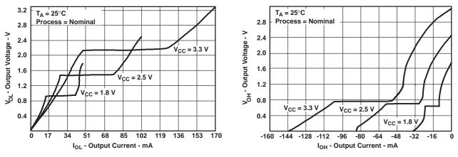
Figure 1. Output Voltage vs Output Current
