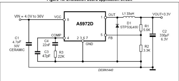
Figure 16. Evaluation board application circuit
