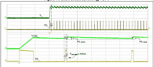
Figure 14. Short-circuit current V<sub>IN</sub> = 24 V
