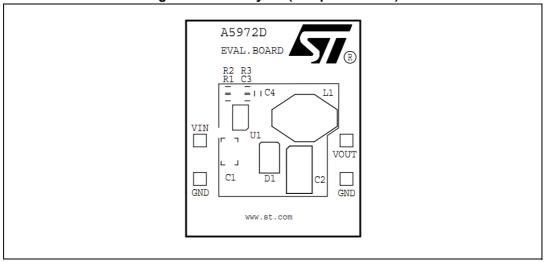
Figure 18. PCB layout (bottom side)
