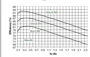
Figure 32. Efficiency vs output current - V<sub>IN</sub> = 12 V
