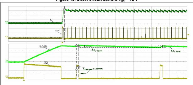
Figure 13. Short-circuit current  $V_{IN}$  = 12 V
