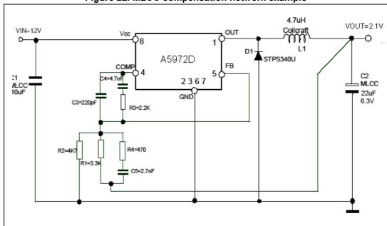
Figure 22. MLCC compensation network example
