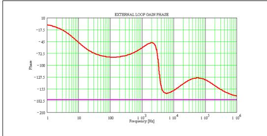
The cut-off frequency and the phase margin are:
