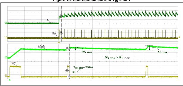
Figure 15. Short-circuit current  $V_{IN} = 36 \text{ V}$
