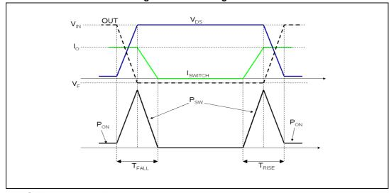
Figure 12. Switching losses
