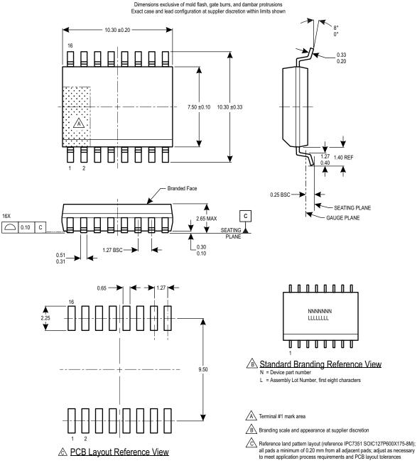
Figure 11: Package MA, 16-pin SOICW
