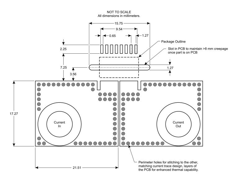
Figure 10: High-Isolation PCB Layout
