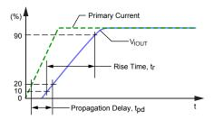
Figure 8: Rise Time and Propagation Delay
