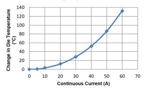
Figure 4: Self-Heating in the MA Package
