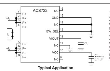
The ACS722 outputs an analog signal, V<sub>IOUT</sub>, that changes, proportionally, with the bidirectional AC or DC primary sensed current, I<sub>P</sub>, within the specified measurement range. The BW\_SEL pin can be used to select one of the two bandwidths to optimize the noise performance. Grounding the BW\_SEL pin puts the part in the high bandwidth (80 kHz) mode.
