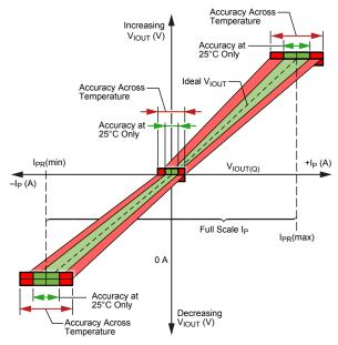
Figure 1: Output Voltage versus Sensed Current
