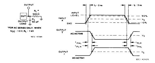
Fig. 3 - Propagation delay times and test circuit.
