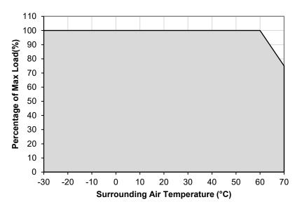
Fig. 1 De-rating for Vertical Mounting Orientation > 60°C de-rate power by 2.5 % / °C
