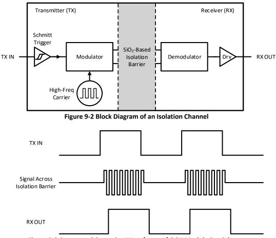
Figure 9-3 Conceptual Operation Waveforms of OOK Modulation Scheme
