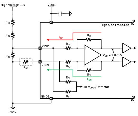
Figure 10-2 Typical Application for Voltage Sensing
