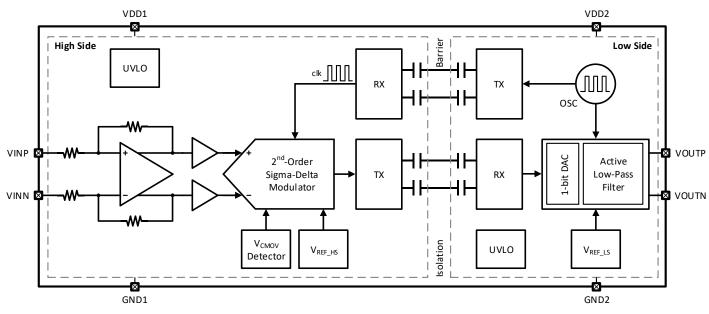
Figure 9-1 Functional Block Diagram of CA-IS1200
