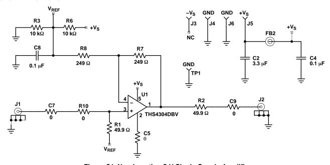
Figure 54. Non-Inverting 5-V Single-Supply Amplifier
