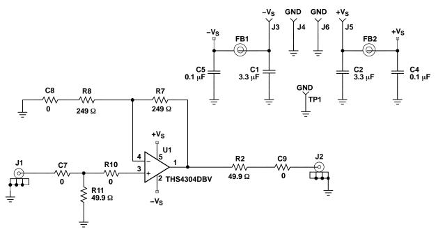
Figure 52. Non-Inverting Gain with Split Power Supply
