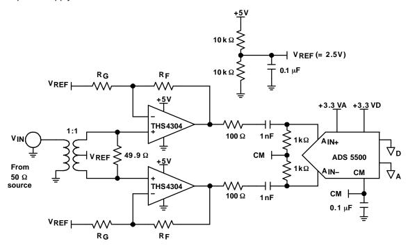
Figure 55. Differential ADC Drive Amplifier Circuit
