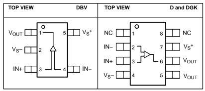
NOTE: NC indicates there is no internal connection to these pins.
