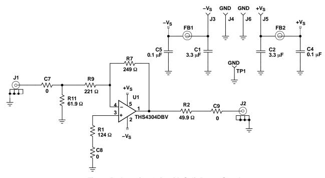
Figure 53. Inverting Gain with Split Power Supply
