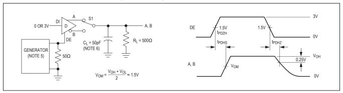
Figure 5. Driver Enable and Disable Times
