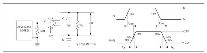
Figure 4. Driver Differential Output Delay and Transition Times
