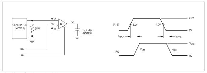
Figure 7. Receiver Propagation Delay
