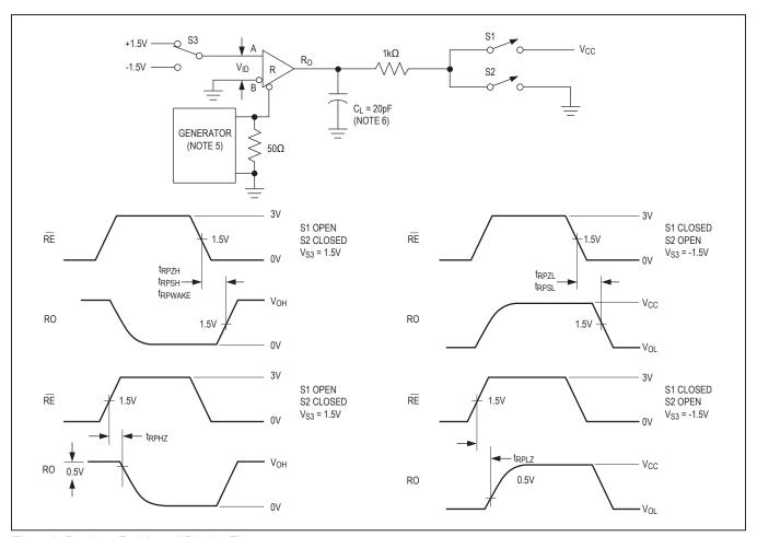
Figure 8. Receiver Enable and Disable Times
