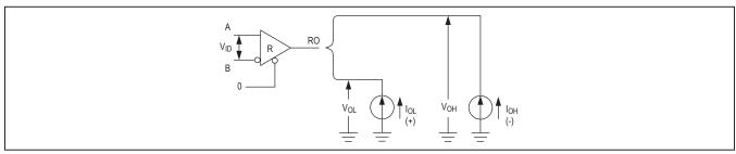
Figure 2. Receiver  $V_{OH}$  and  $V_{OL}$
