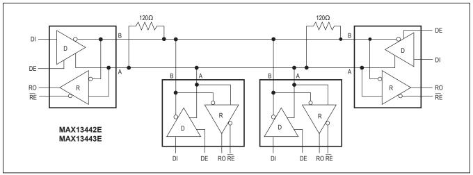
Figure 13. MAX13442E/MAX13443E Typical RS-485 Network
