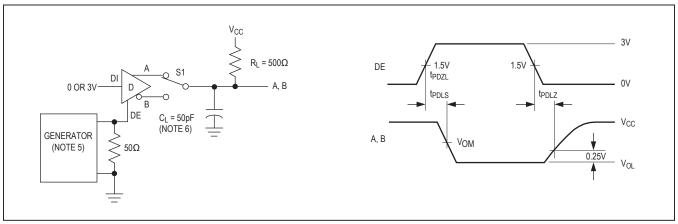
Figure 6. Driver Enable and Disable Times
