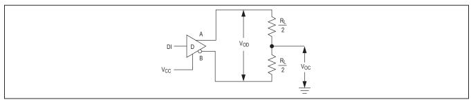
Figure 1. Driver V<sub>OD</sub> and V<sub>OC</sub>
