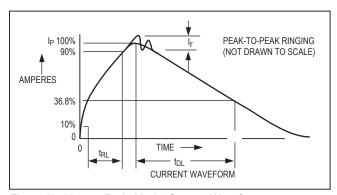
Figure 9b. Human Body Model Current Waveform
