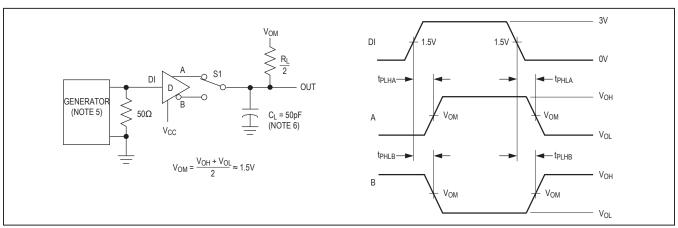
Figure 3. Driver Propagation Times
