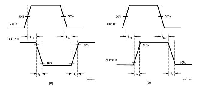
FIGURE 1. (a) Inverting, (b) Non-Inverting
