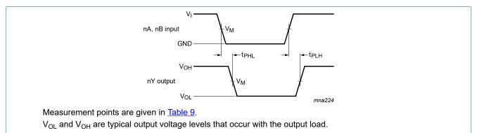
Fig. 6. Input (nA, nB) to output (nY) propagation delays
